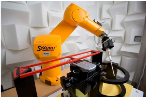
Figure 4-3 SPEAG Robotic System
