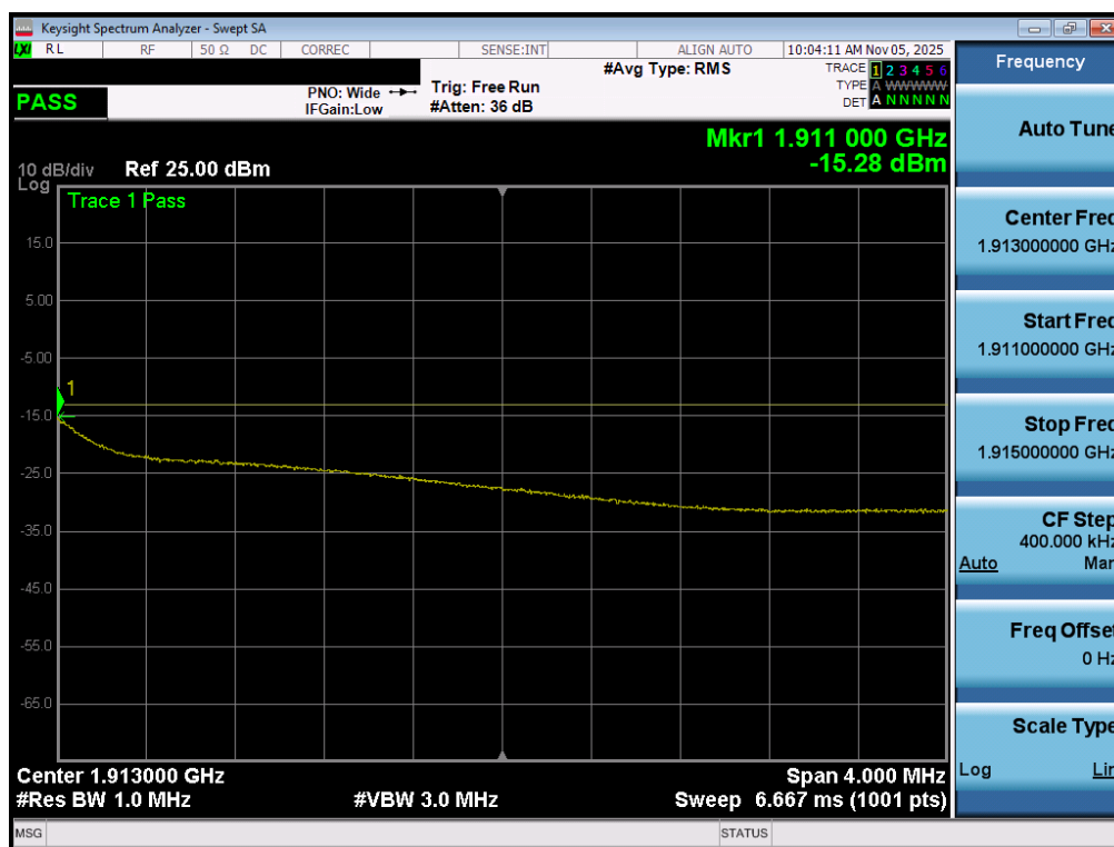
Plot 7-95. Extended Upper Band Edge Plot (WCDMA PCS – Ch. 9538 - Ant1)
