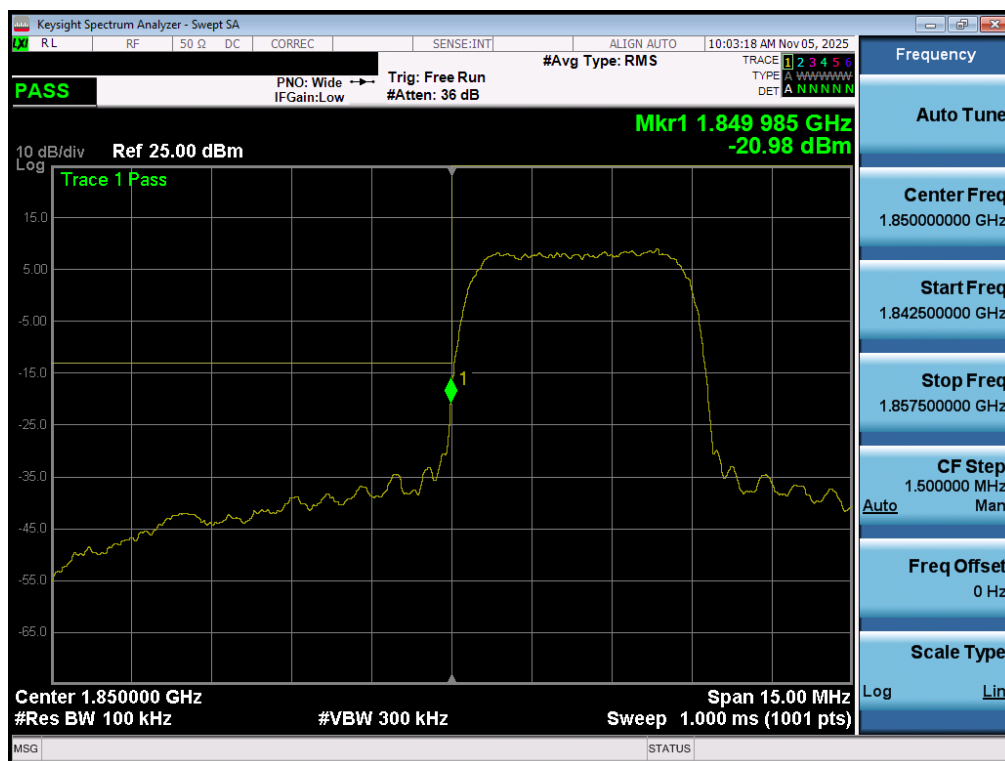
Plot 7-92. Lower Band Edge Plot (WCDMA PCS – Ch. 9262 - Ant1)
