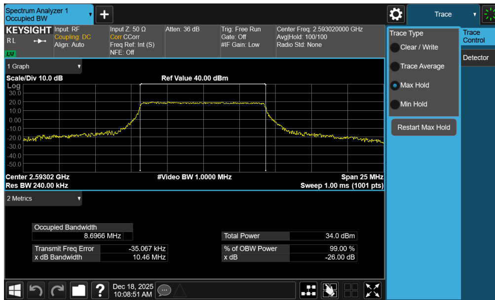
Plot 7-59. Occupied Bandwidth Plot (NR Band n41 PC2 – 10MHz 16-QAM – Full RB – Ant1)
