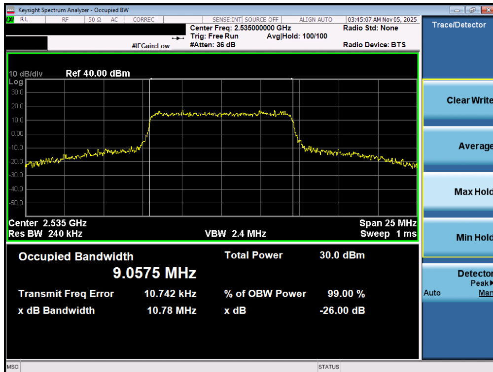
Plot 7-10. Occupied Bandwidth Plot (LTE Band 7 - 10MHz 16-QAM - Full RB - Ant1)
