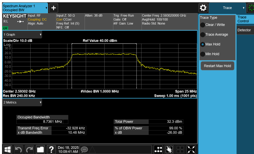
Plot 7-58. Occupied Bandwidth Plot (NR Band n41 PC2 – 10MHz QPSK – Full RB – Ant1)
