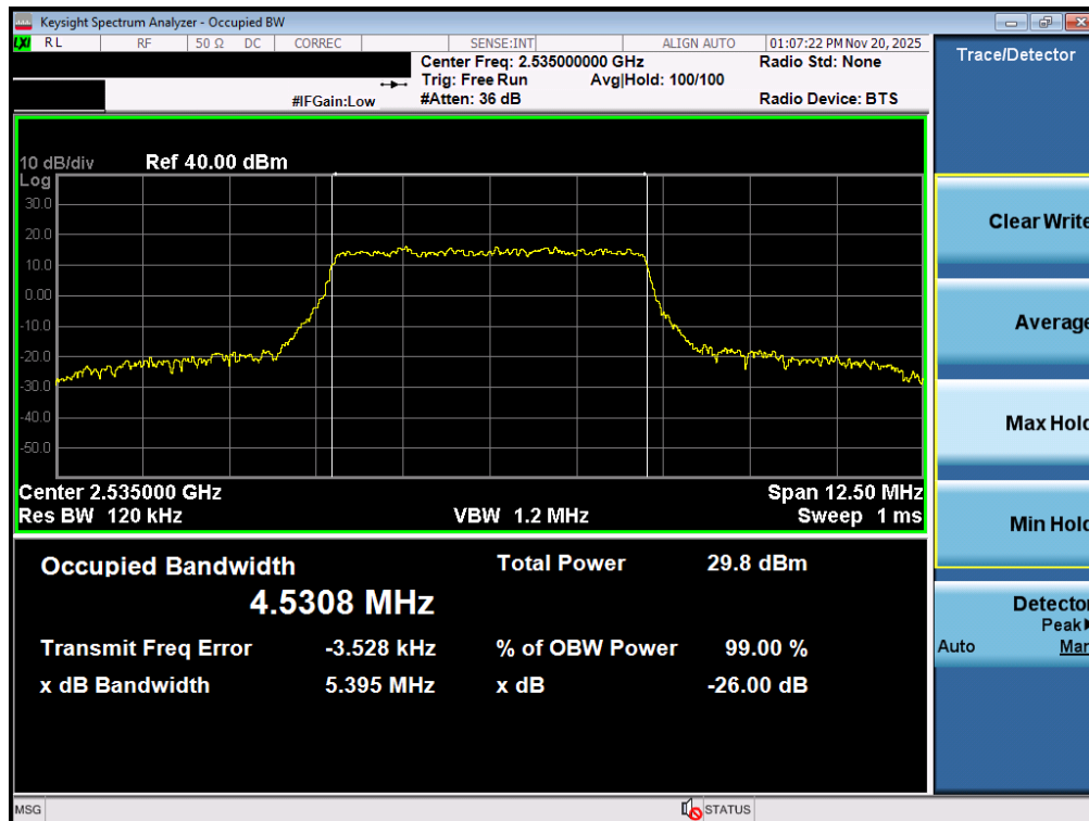
Plot 7-71. Occupied Bandwidth Plot (LTE Band 7 - 5MHz 16-QAM - Full RB - Ant2)
