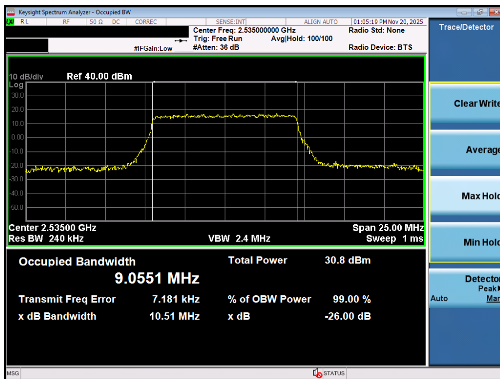
Plot 7-68. Occupied Bandwidth Plot (LTE Band 7 - 10MHz QPSK - Full RB - Ant2)
