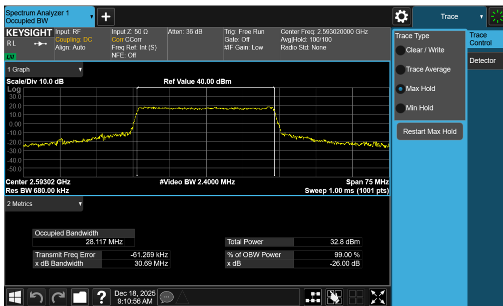
Plot 7-50. Occupied Bandwidth Plot (NR Band n41 PC2 – 30MHz 16-QAM – Full RB – Ant1)
