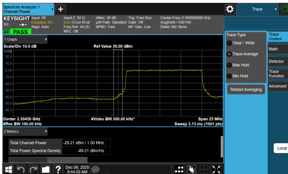
Plot 7-136. Lower Band Edge Plot (LTE Band 30 - 10MHz QPSK – Full RB - Ant2)
