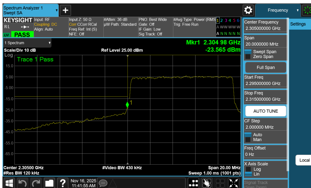
Plot 7-126. Lower Band Edge Plot (NR Band n30 - 10MHz CP-OFDM-QPSK – Full RB - Ant1)
