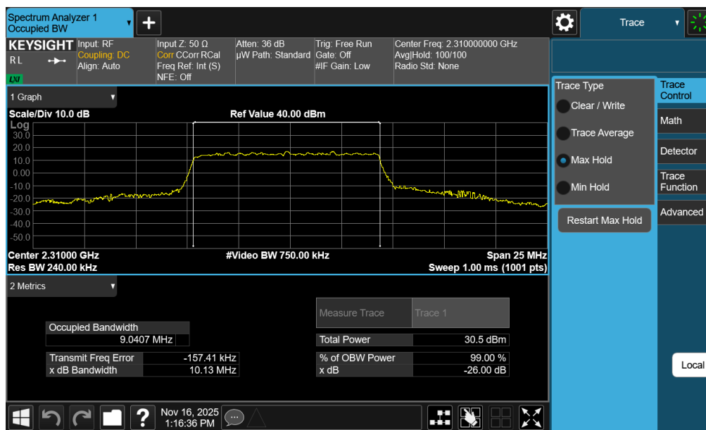
Plot 7-81. Occupied Bandwidth Plot (NR Band n30 - 10MHz QPSK - Full RB - Ant2)
