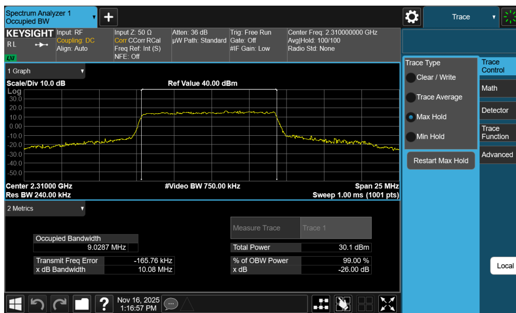
Plot 7-82. Occupied Bandwidth Plot (NR Band n30 - 10MHz 16-QAM - Full RB - Ant2)
