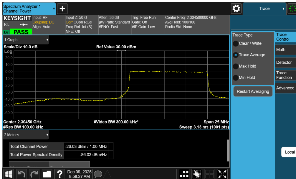
Plot 7-114. Lower Band Edge Plot (LTE Band 30 - 10MHz QPSK – Full RB - Ant1)
