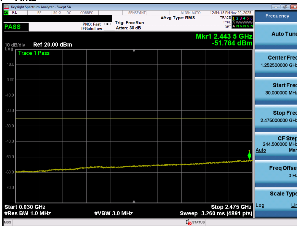
Plot 7-107. Conducted Spurious Plot (LTE Band 7 - 20MHz QPSK - RB Size 1, RB Offset 0 - Low Channel - Ant2)
