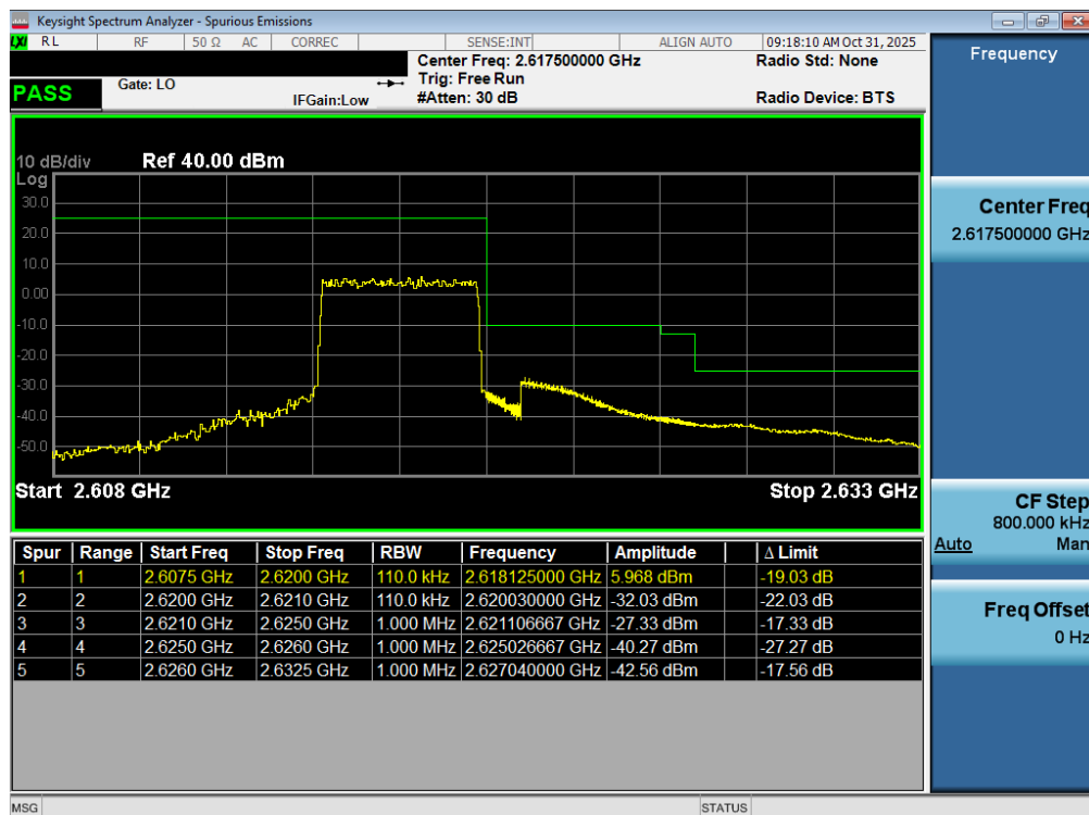
Plot 7-123. Upper ACP Plot (LTE Band 38 - 5MHz QPSK – Full RB - Ant1)
