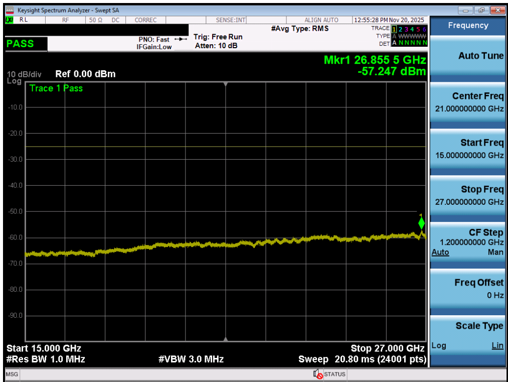
Plot 7-109. Conducted Spurious Plot (LTE Band 7 - 20MHz QPSK - RB Size 1, RB Offset 0 - Low Channel - Ant2)
