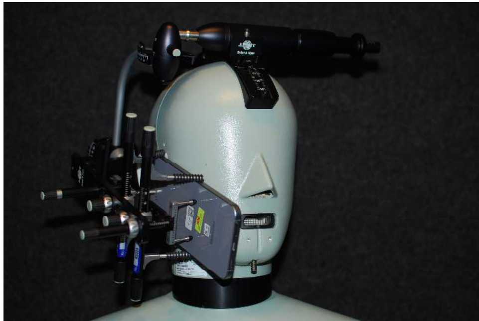
Figure 17-4 Test Setup for Wireless Device
