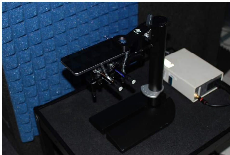
Figure 17-1 Wireless Device in Handset Positioner
