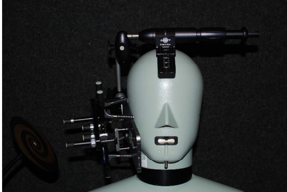
Figure 17-3 Test Setup for Wireless Device
