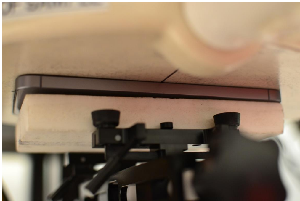
SAR Test Setup Photo 10 – Phablet, Front Side at 0mm
