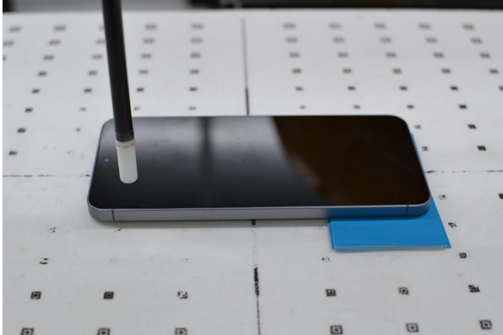
PD Test Setup Photo 30 – PD, Front Side at 10.07mm (Antenna G)
