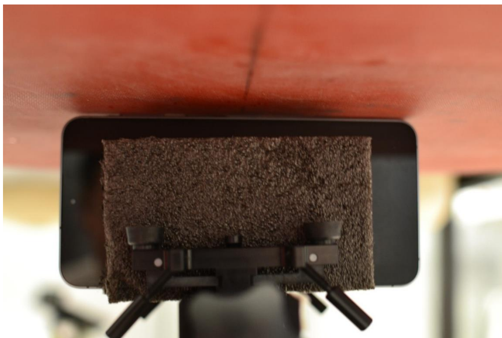
SAR Test Setup Photo 20 – NFC Phablet, Right Edge at 0mm
