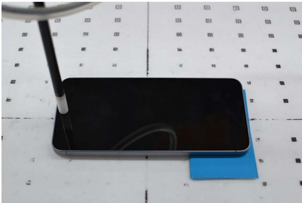
PD Test Setup Photo 29 – PD, Front Side at 2mm (MIMO)
