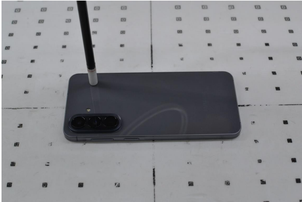
PD Test Setup Photo 25 – PD, Back Side at 2mm (Antenna G)
