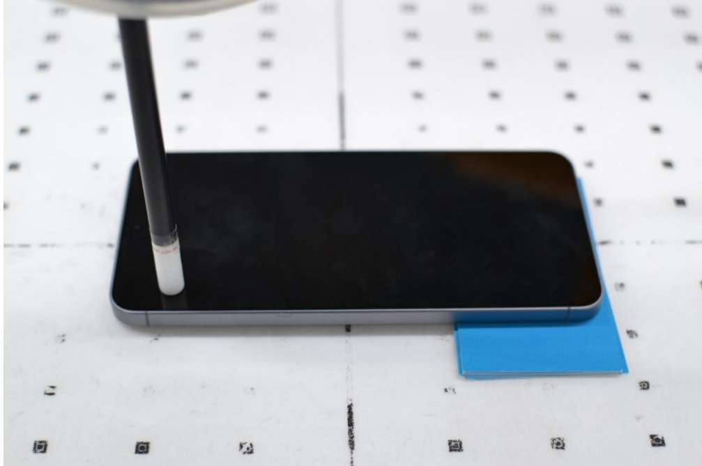
PD Test Setup Photo 28 – PD, Front Side at 2mm (Antenna G)
