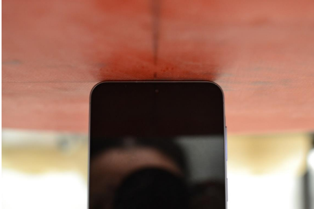
SAR Test Setup Photo 17 – NFC Phablet, Top Edge at 0mm
