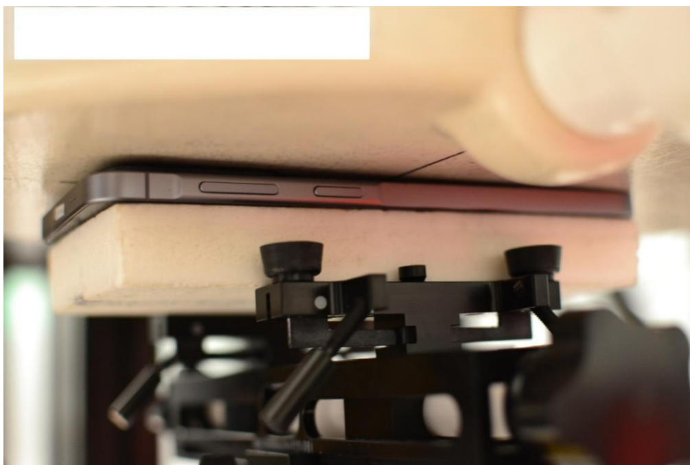
SAR Test Setup Photo 6 – Phablet, Back Side at 0mm (for AG0 bands)
