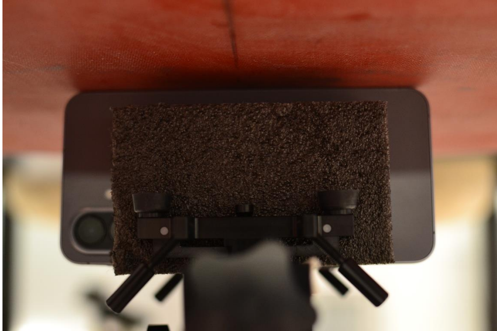
SAR Test Setup Photo 23 – NFC Phablet, Left Edge at 0mm
