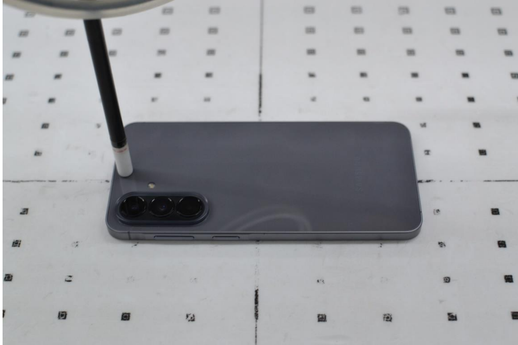
PD Test Setup Photo 26 – PD, Back Side at 2mm (MIMO)
