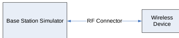
Figure 9-2 Power Measurement Setup
