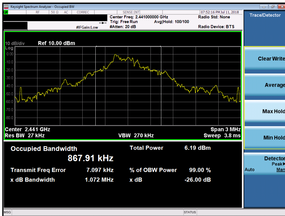
Plot 7-1. Occupied Bandwidth Plot (ANT+ – Ch. 39)
