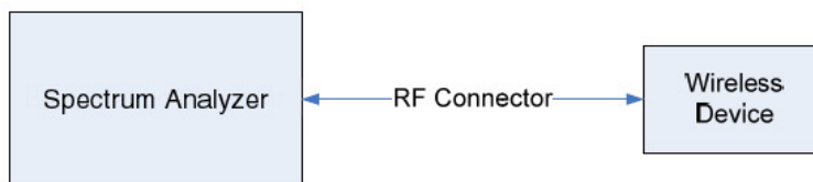
Figure 7-1. Test Instrument & Measurement Setup
