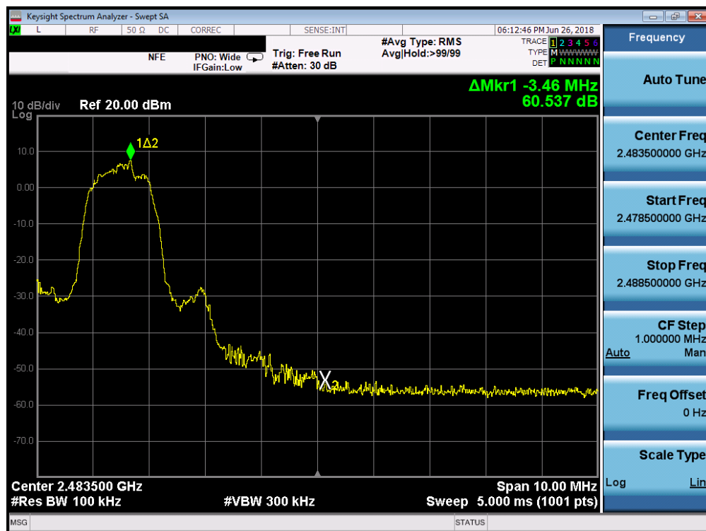
Plot 7-29. Band Edge Plot (Bluetooth with Hopping Disabled, 3 Mbps – Ch. 78)
