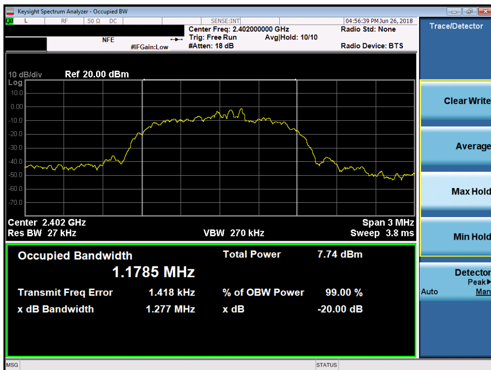
Plot 7-7. 20dB Bandwidth Plot (Bluetooth, 3Mbps – Ch. 0)
