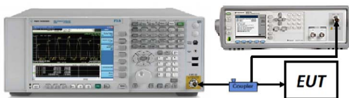
Figure 7-6. Test Instrument & Measurement Setup
