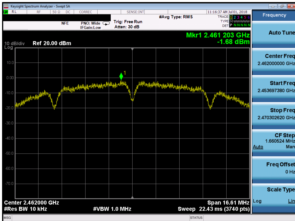
Plot 7-12. Power Spectral Density Plot (802.11b – Ch. 11)
