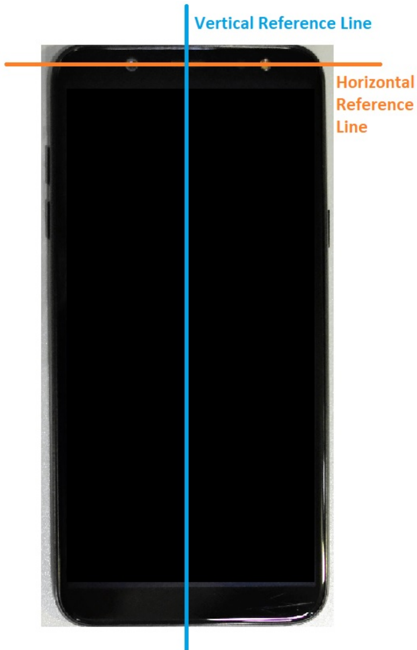
SAR Test Setup Photo 13 – Horizontal and Vertical Reference Lines
