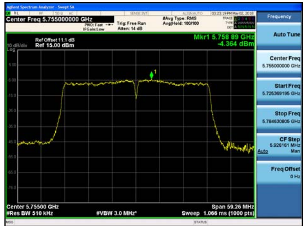
802.11n_HT40 UNII 3 BAND PSD CH 151
