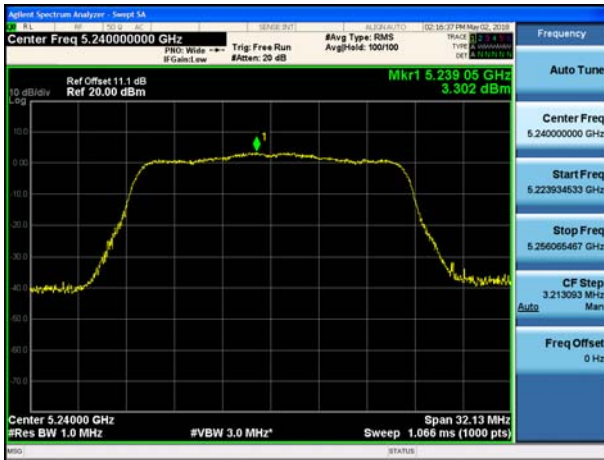
802.11n_HT20 UNII 2C BAND PSD CH 100
