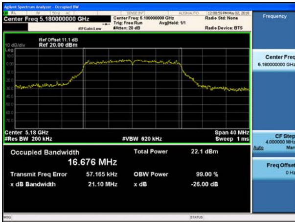
802.11a UNII 2C BAND 26dB Bandwidth (CH100)
