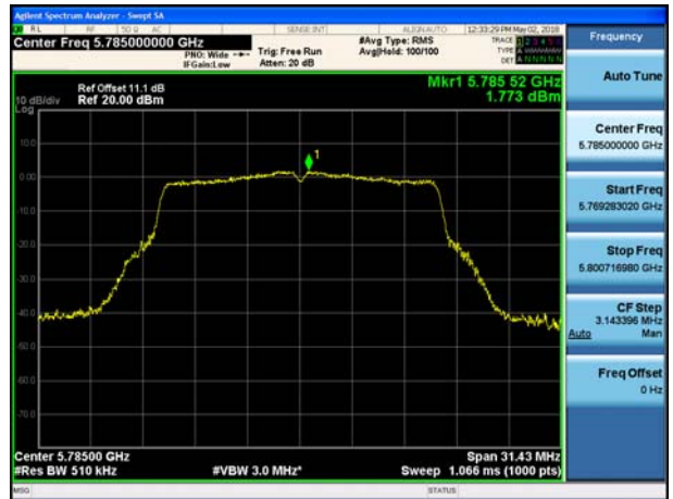
802.11a UNII 3 BAND PSD CH 157
