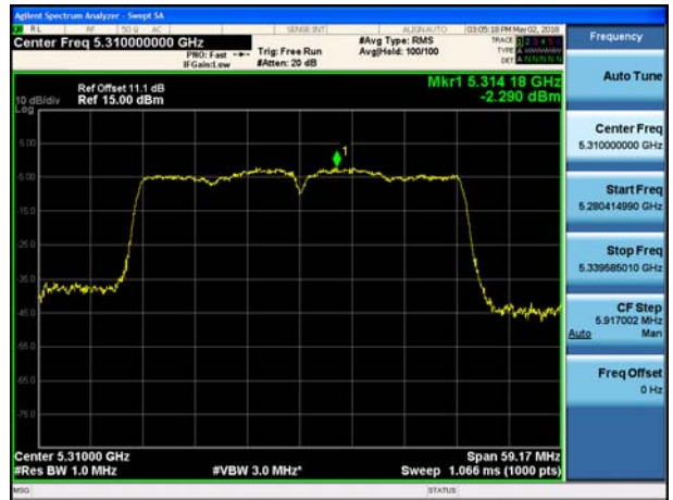
802.11n_HT40 UNII 3 BAND PSD CH 151
