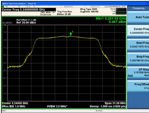
802.11a UNII 2C BAND PSD CH 140
