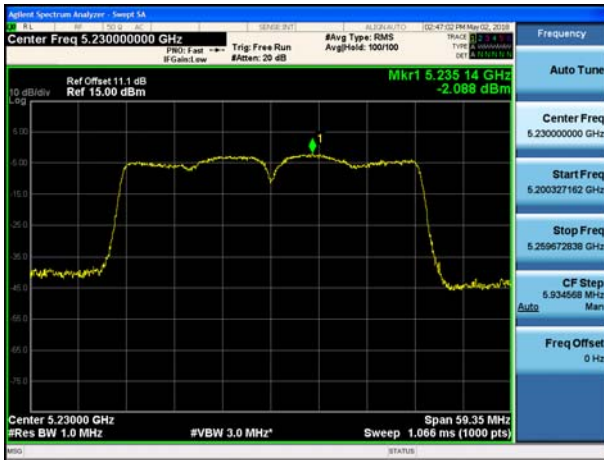
802.11n_HT40 UNII 2C BAND PSD CH 134
