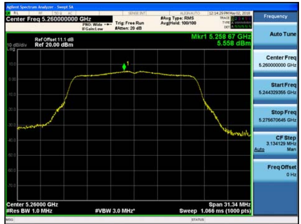
802.11a UNII 3 BAND PSD CH 157
