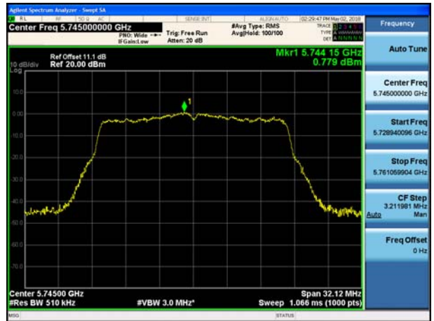
802.11n_HT20 UNII 3 BAND PSD CH 149
