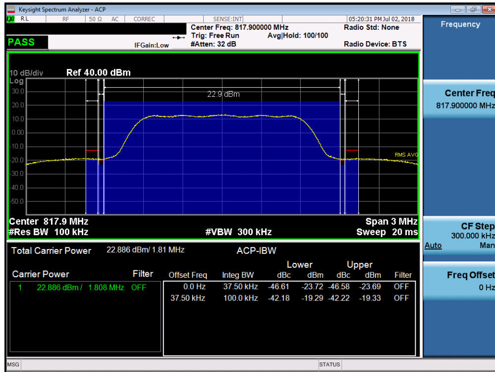
Plot 7-22. Channel Edge Plot (CDMA BC10 - Ch. 476)
