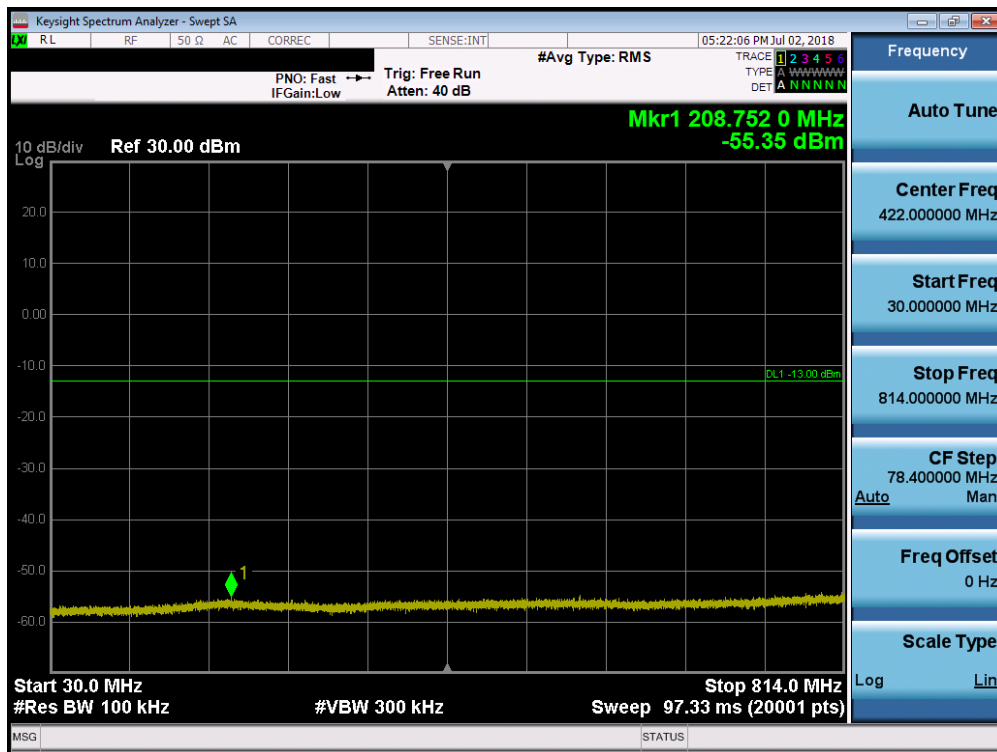
Plot 7-16. Conducted Spurious Plot (CDMA – Ch. 684)
