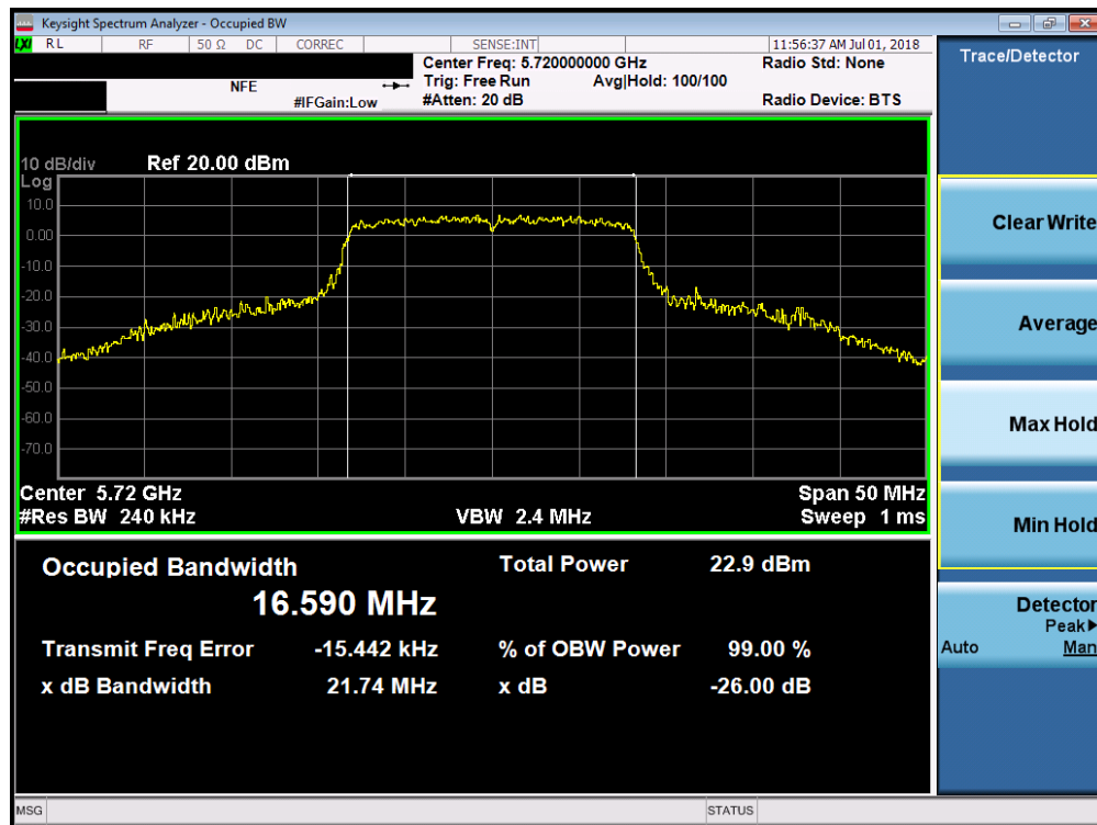
Plot 7-21. 26dB Bandwidth Plot (802.11a (UNII Band 2C) – Ch. 144)
