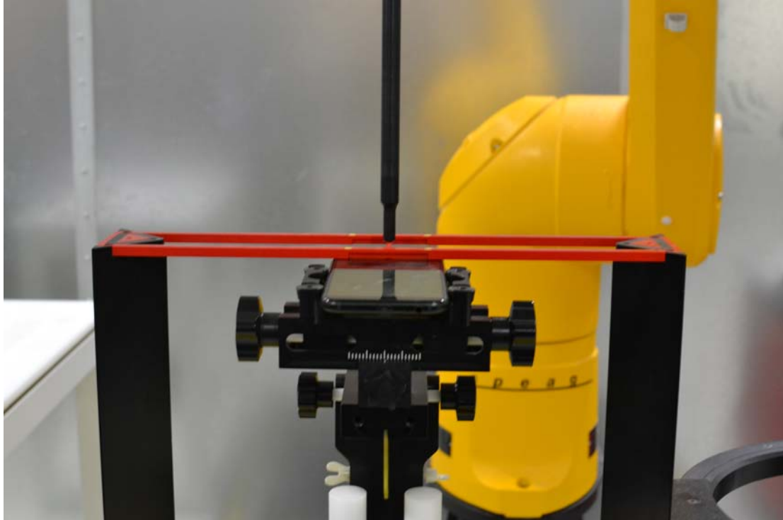
Figure 18-1 Ear Reference Point HAC Phantom Alignment
