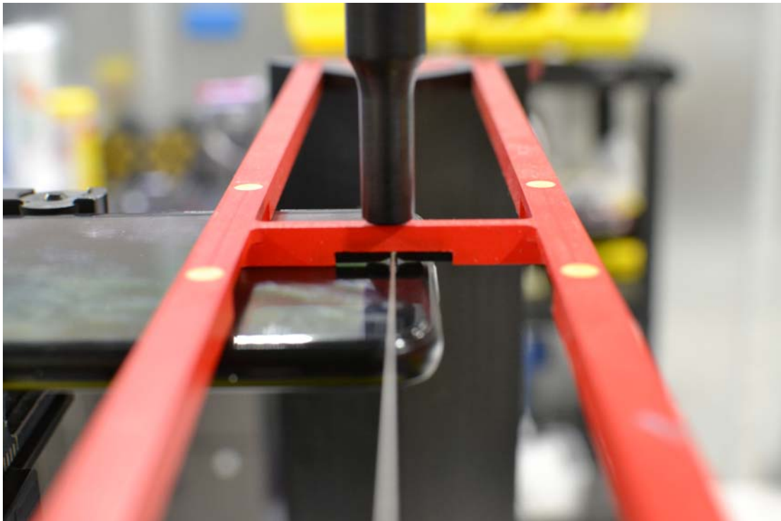
Figure 18-2 HAC Phantom Plane Alignment
