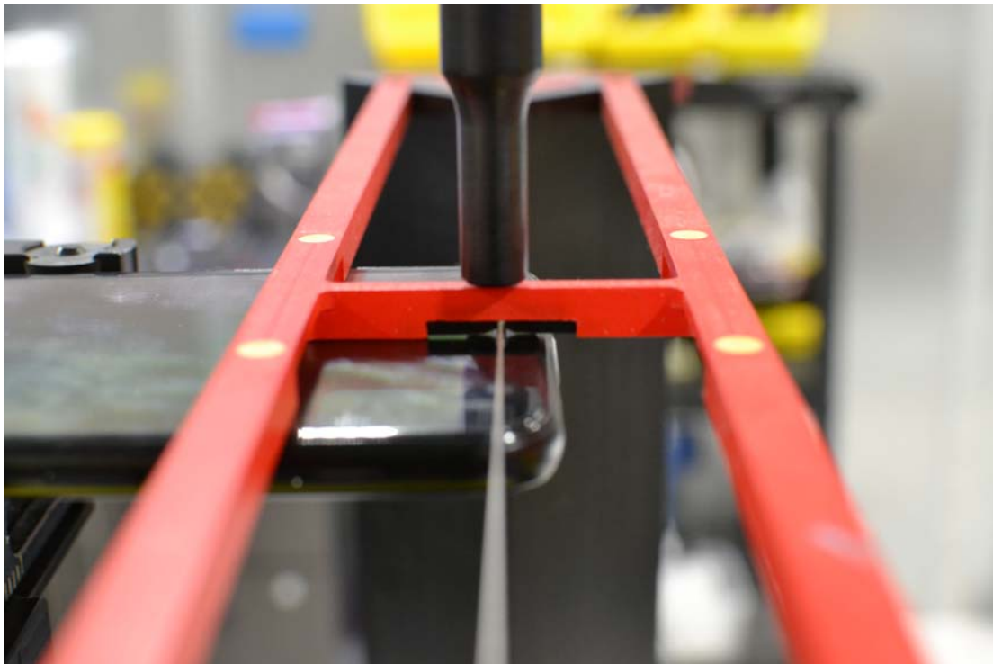
Figure 18-2 HAC Phantom Plane Alignment
