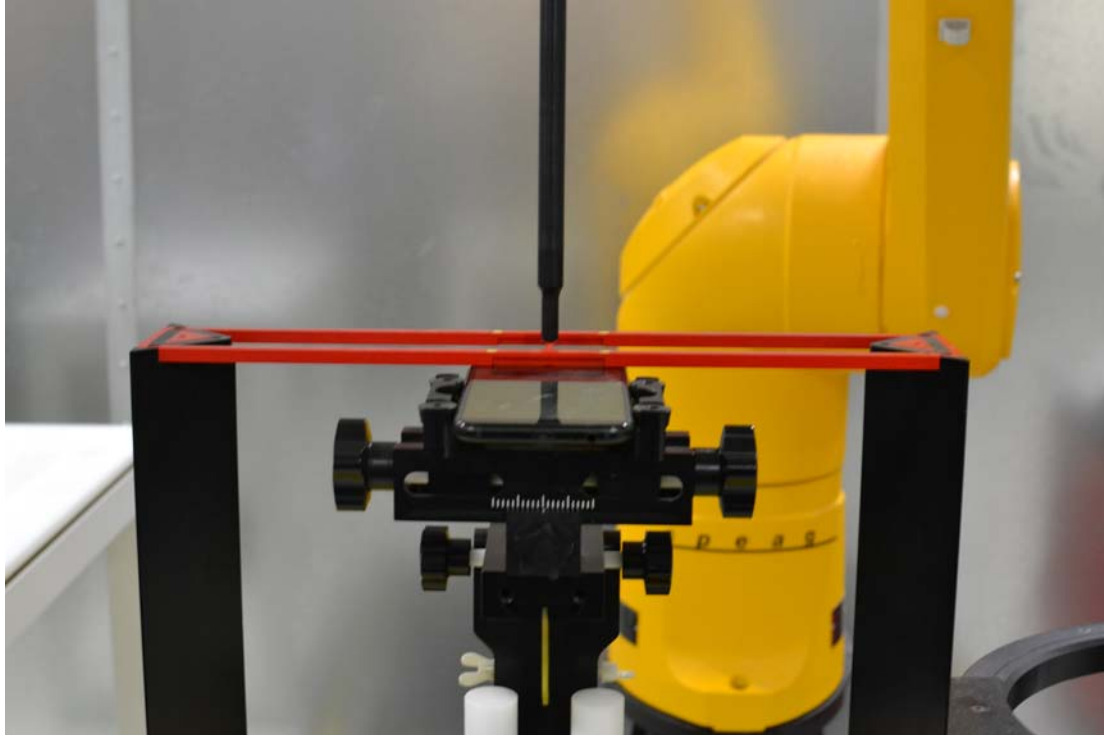
Figure 18-1 Ear Reference Point HAC Phantom Alignment
