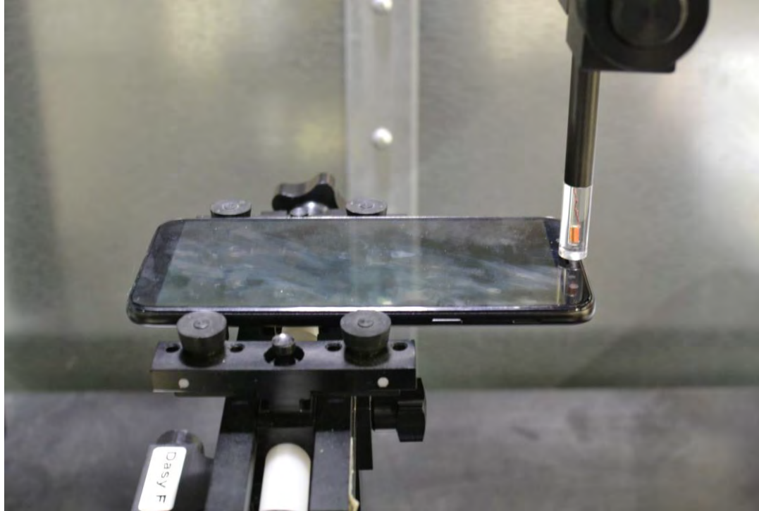
Figure 16-1 Test Setup for Wireless Device
