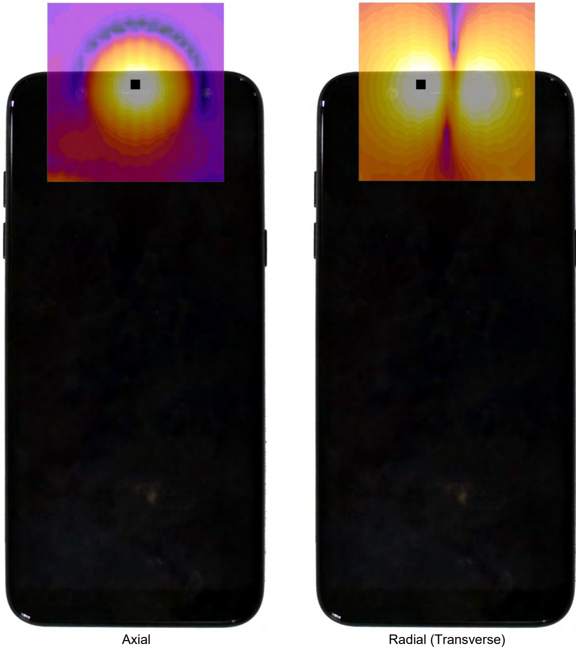
Figure 16-3 T-Coil Scan Overlay Magnetic Field Distributions
