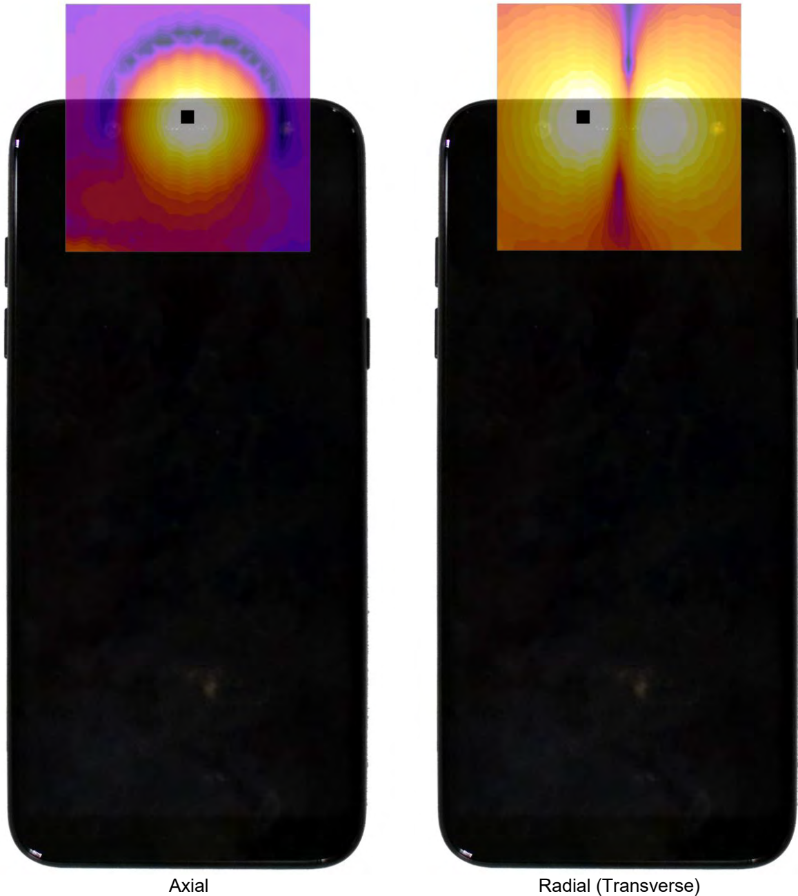
Figure 16-3 T-Coil Scan Overlay Magnetic Field Distributions
