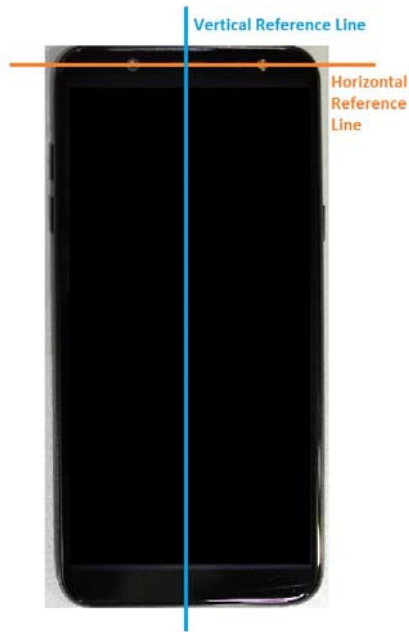
SAR Test Setup Photo 13: Vertical and Horizontal Reference Lines
