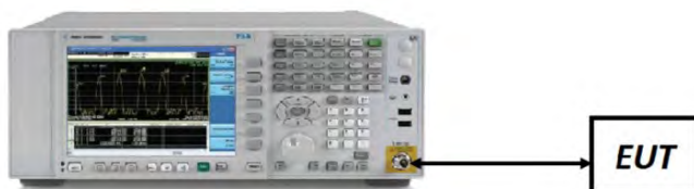
Figure 7-2. Test Instrument & Measurement Setup
