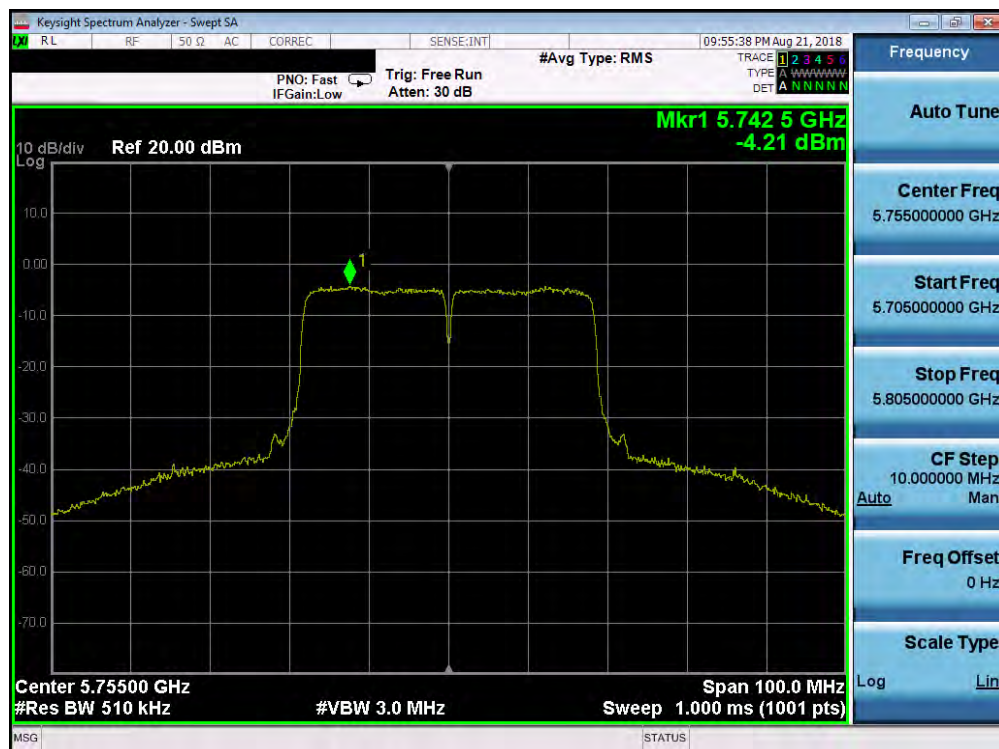
Plot 7-76. Power Spectral Density Plot (40MHz BW 802.11n (UNII Band 3) – Ch. 151)
