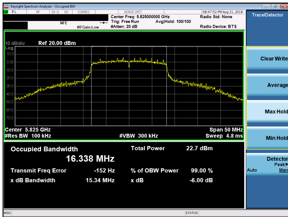
Plot 7-33. 6dB Bandwidth Plot (802.11a (UNII Band 3) – Ch. 165)
