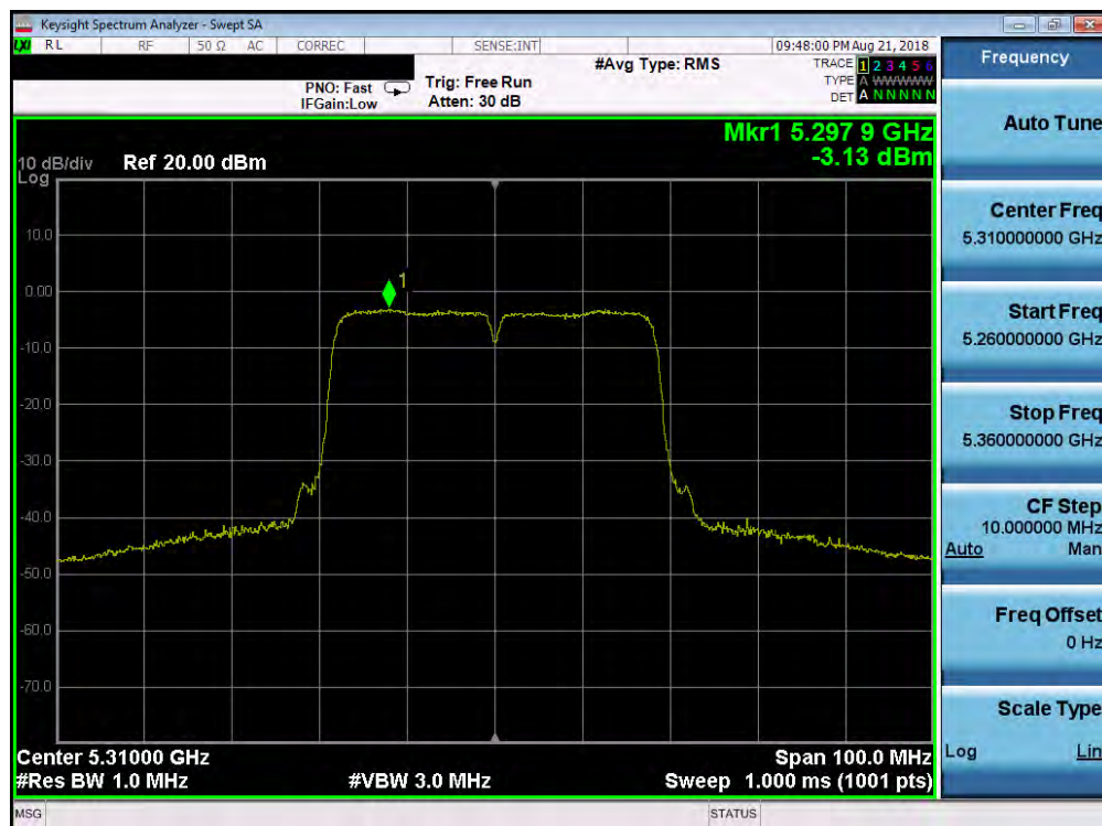
Plot 7-56. Power Spectral Density Plot (40MHz BW 802.11n (UNII Band 2A) – Ch. 62)
