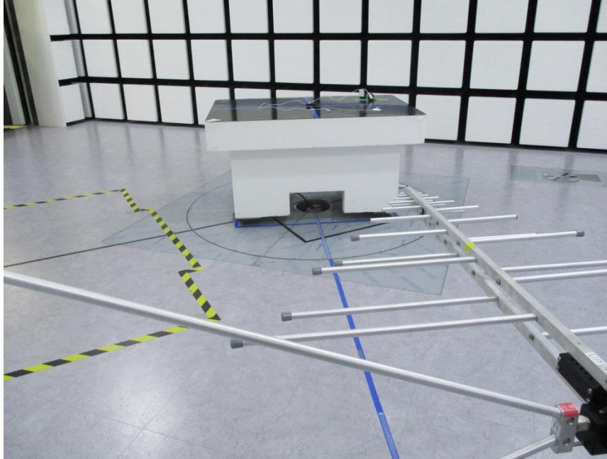
RADIATED FRONT PHOTO (BELOW 1 GHz)
