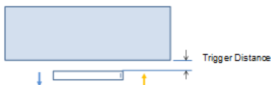
Proximity Sensor Trigger Distance Assessment KDB 616217 §6.2, Front
