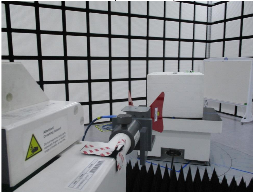
RADIATED FRONT PHOTO (ABOVE 1 GHz)
