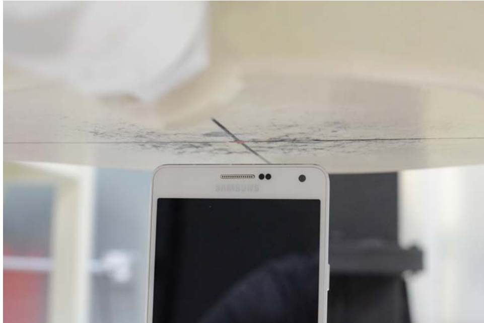
SAR Test Setup Photo 7: Top at 1.0 cm
