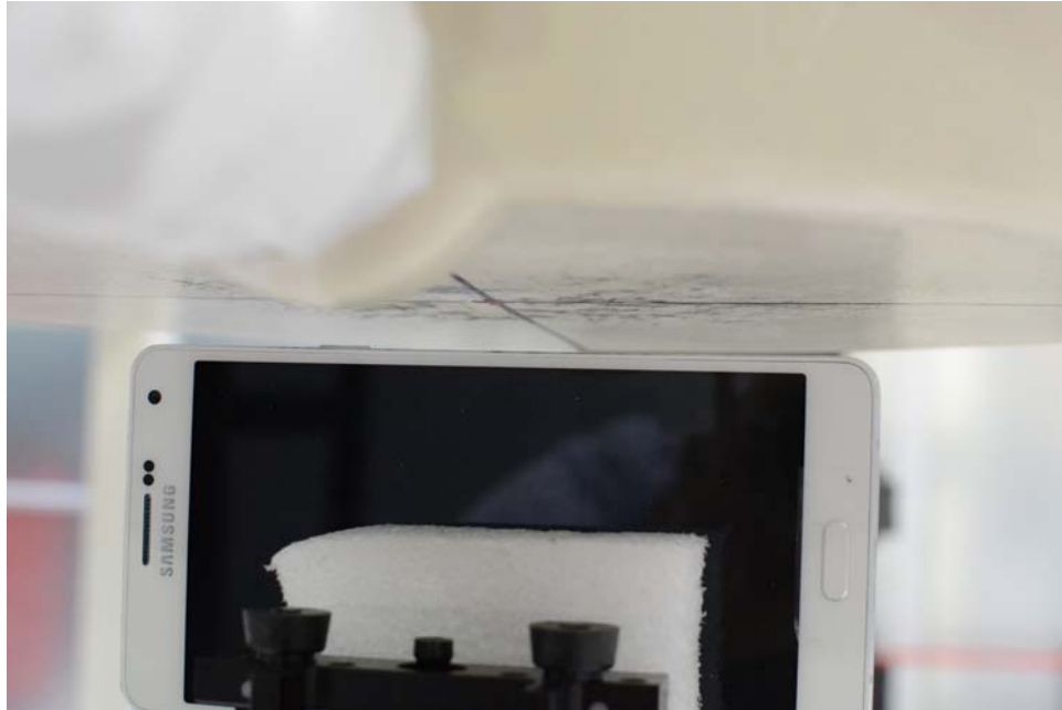
SAR Test Setup Photo 9: Right at 1.0 cm
