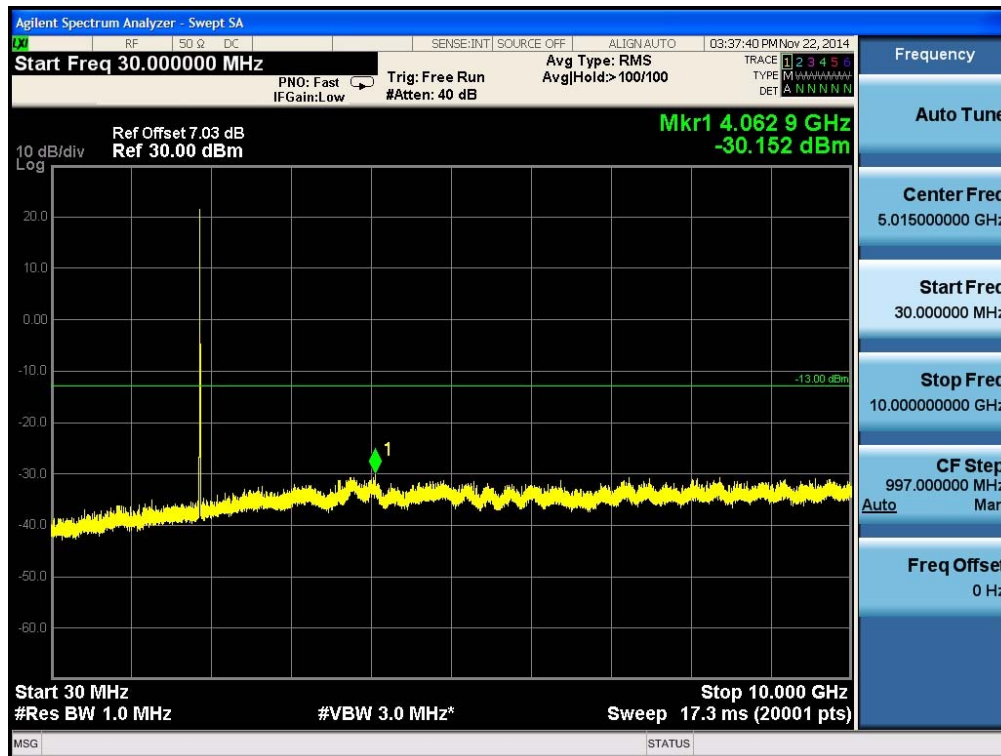
Plot 6-27. Conducted Spurious Plot (PCS WCDMA Mode - Ch.9400(DL9800))
