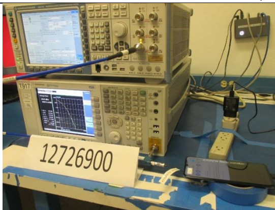
ANTENNA PORT CONDUCTED PHOTO
