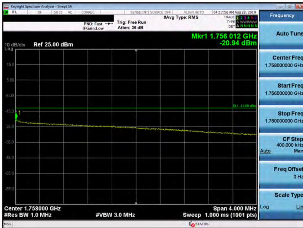
Plot 7-143. Upper Extended Band Edge Plot (Band 4 - 10.0MHz QPSK - Full RB Configuration)
