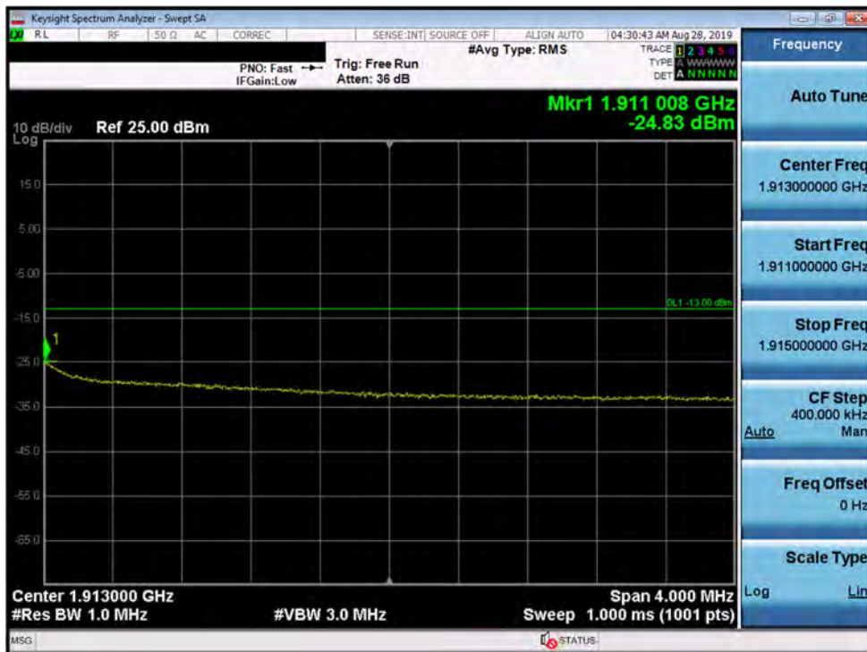
Plot 7-173. Upper Extended Band Edge Plot (Band 2 - 10.0MHz QPSK - Full RB Configuration)
