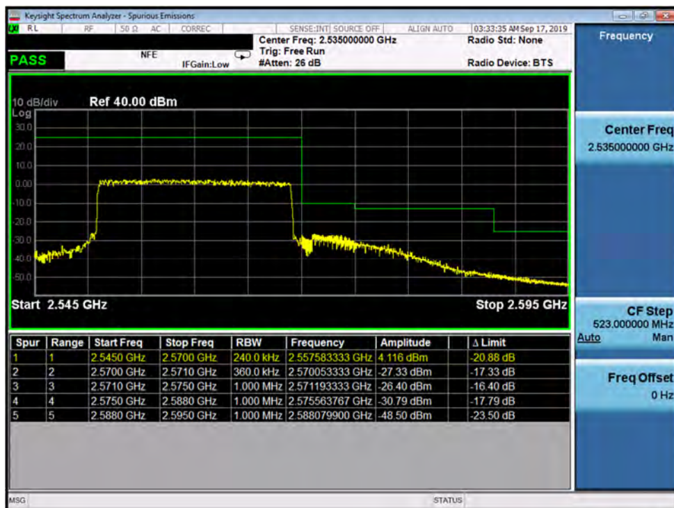
Plot 7-189. Upper ACP Plot (Band 7 - 20.0MHz QPSK - Full RB Configuration)
