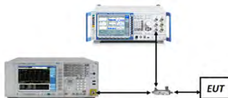
Figure 7-4. Test Instrument & Measurement Setup
