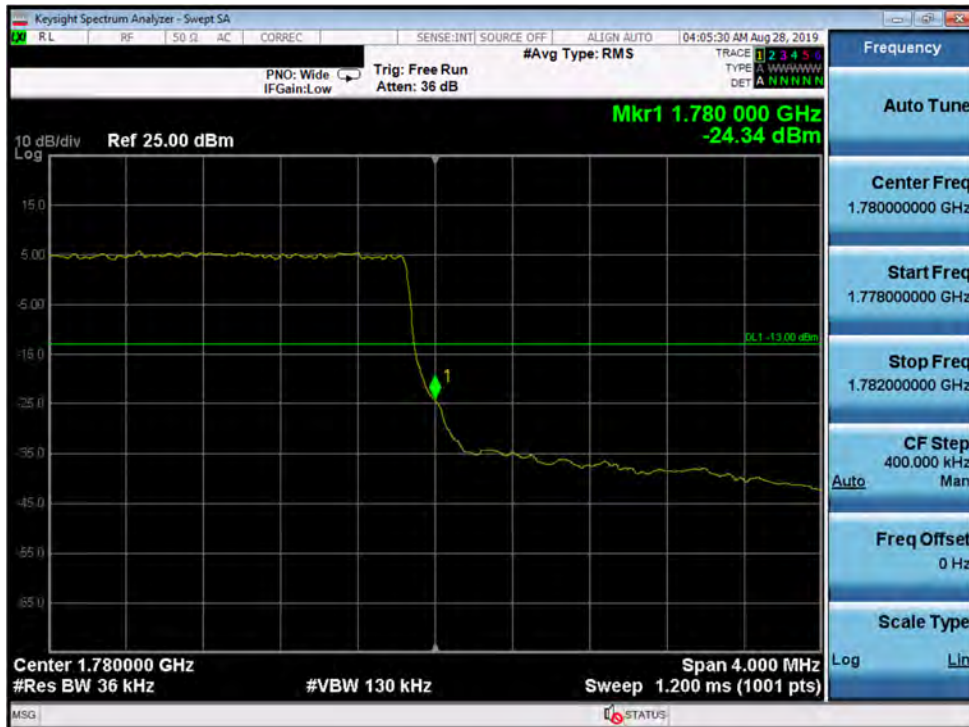
Plot 7-132. Upper Band Edge Plot (Band 66 - 3.0MHz QPSK - Full RB Configuration)
