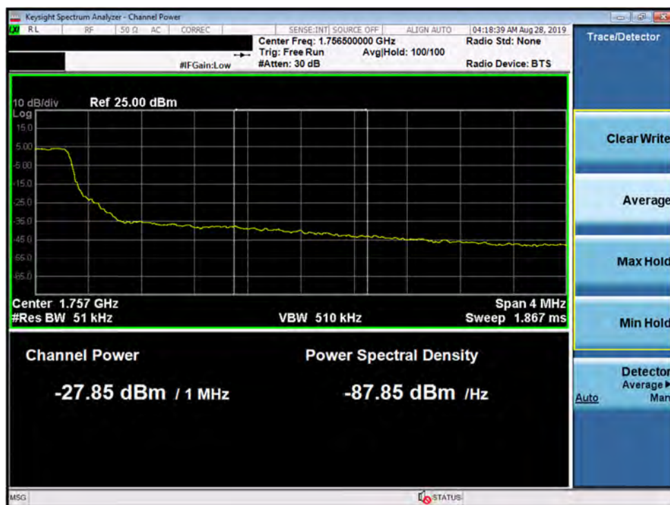
Plot 7-137. Upper Extended Band Edge Plot (Band 4 - 5.0MHz QPSK - Full RB Configuration)
