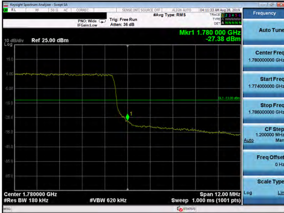
Plot 7-150. Upper Band Edge Plot (Band 66 - 15.0MHz QPSK - Full RB Configuration)
