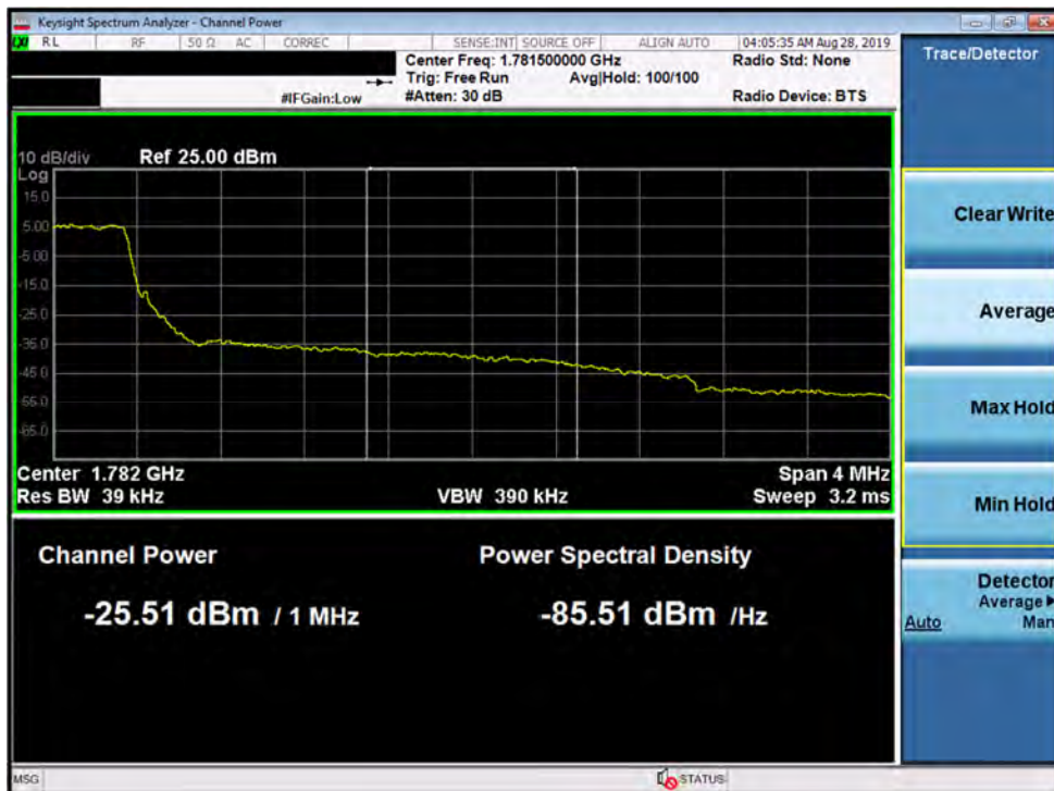
Plot 7-133. Upper Extended Band Edge Plot (Band 66 - 3.0MHz QPSK - Full RB Configuration)
