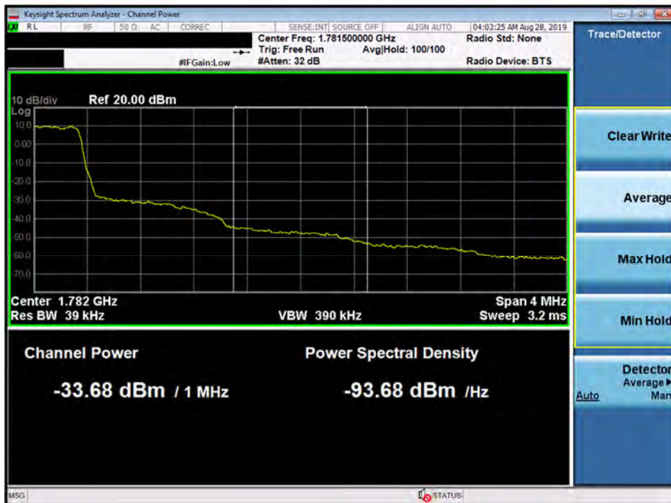
Plot 7-127. Upper Extended Band Edge Plot (Band 66 - 1.4MHz QPSK - Full RB Configuration)
