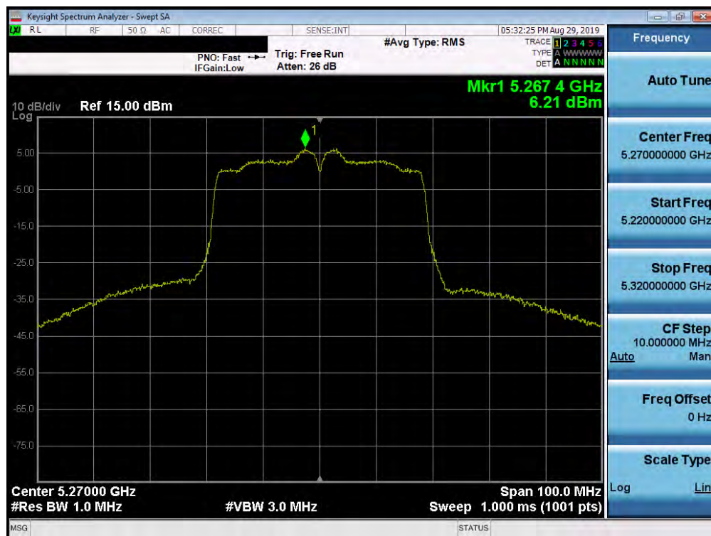
Plot 7-55. Power Spectral Density Plot (40MHz BW 802.11n (UNII Band 2A) – Ch. 54)
