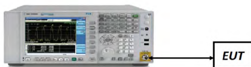
Figure 7-4. Test Instrument & Measurement Setup
