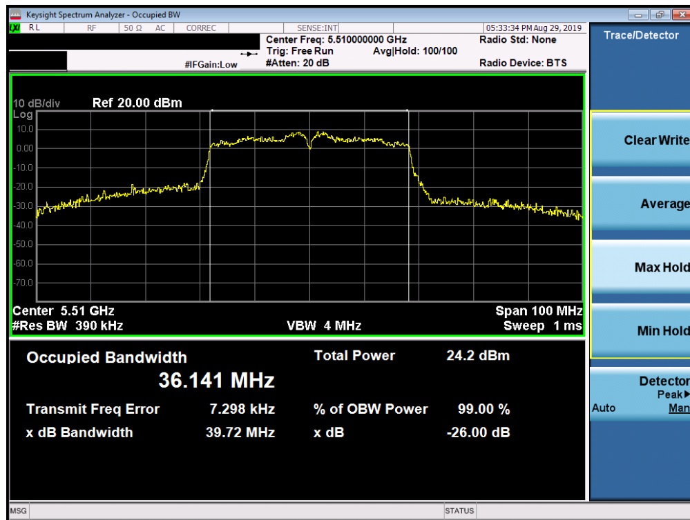
Plot 7-25. 26dB Bandwidth Plot (40MHz BW 802.11n (UNII Band 2C) – Ch. 102)
