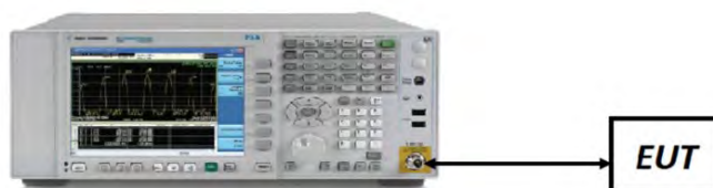
Figure 7-2. Test Instrument & Measurement Setup
