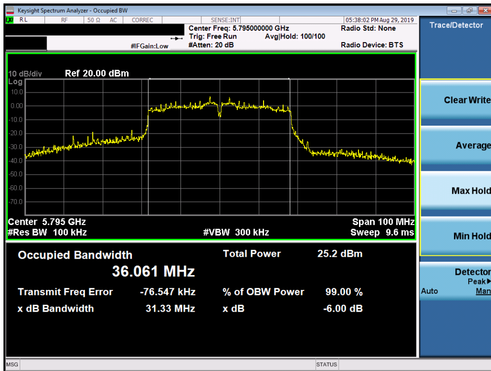
Plot 7-38. 6dB Bandwidth Plot (40MHz BW 802.11n (UNII Band 3) – Ch. 159)
