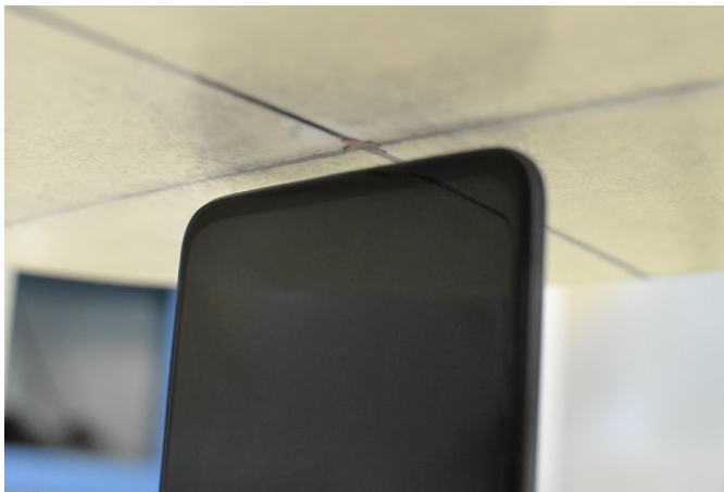
SAR Test Setup Photo 14 – Bottom Edge at 4 mm
