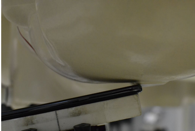
SAR Test Setup Photo 4 – Left Tilt
