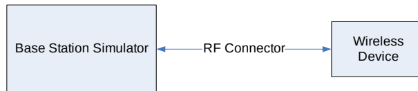
Figure 9-3 Power Measurement Setup
