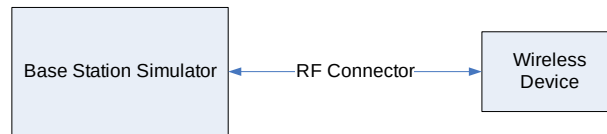
Figure 9-1 Power Measurement Setup
