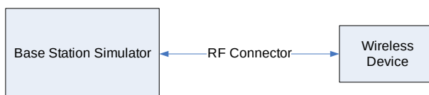
Figure 9-2 Power Measurement Setup
