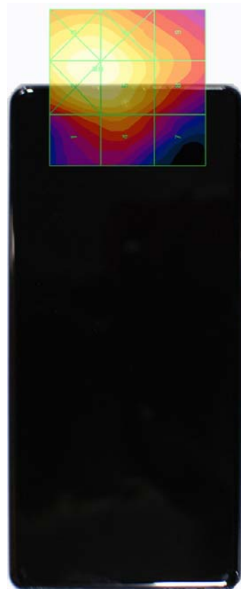
Figure 18-4 E-Field WD Scan overlay
