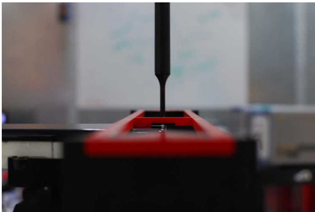
Figure 18-2 HAC Phantom Plane Alignment
