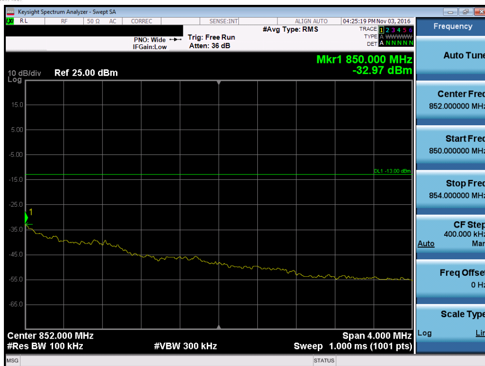
Plot 7-99. Upper Extended Band Edge Plot (Band 5 – 1.4MHz QPSK – RB Size 6)
