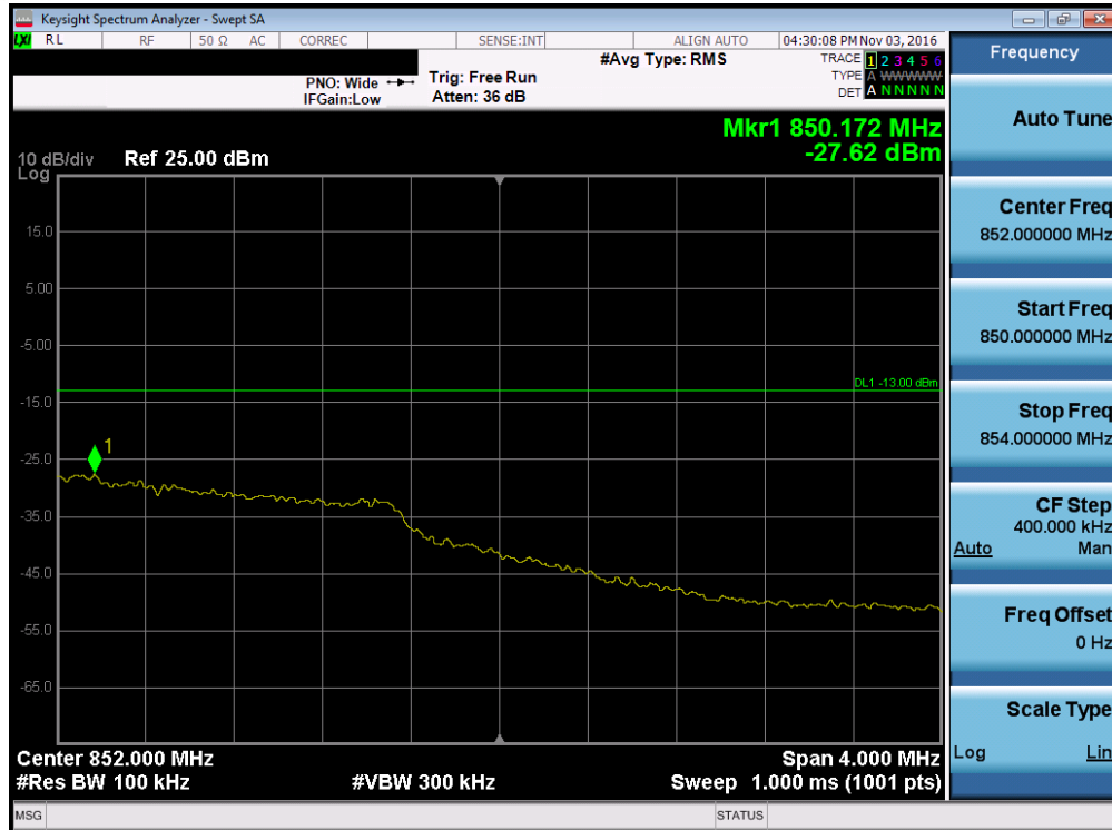
Plot 7-103. Upper Extended Band Edge Plot (Band 5 – Band 5 – 3.0MHz QPSK – RB Size 15)
