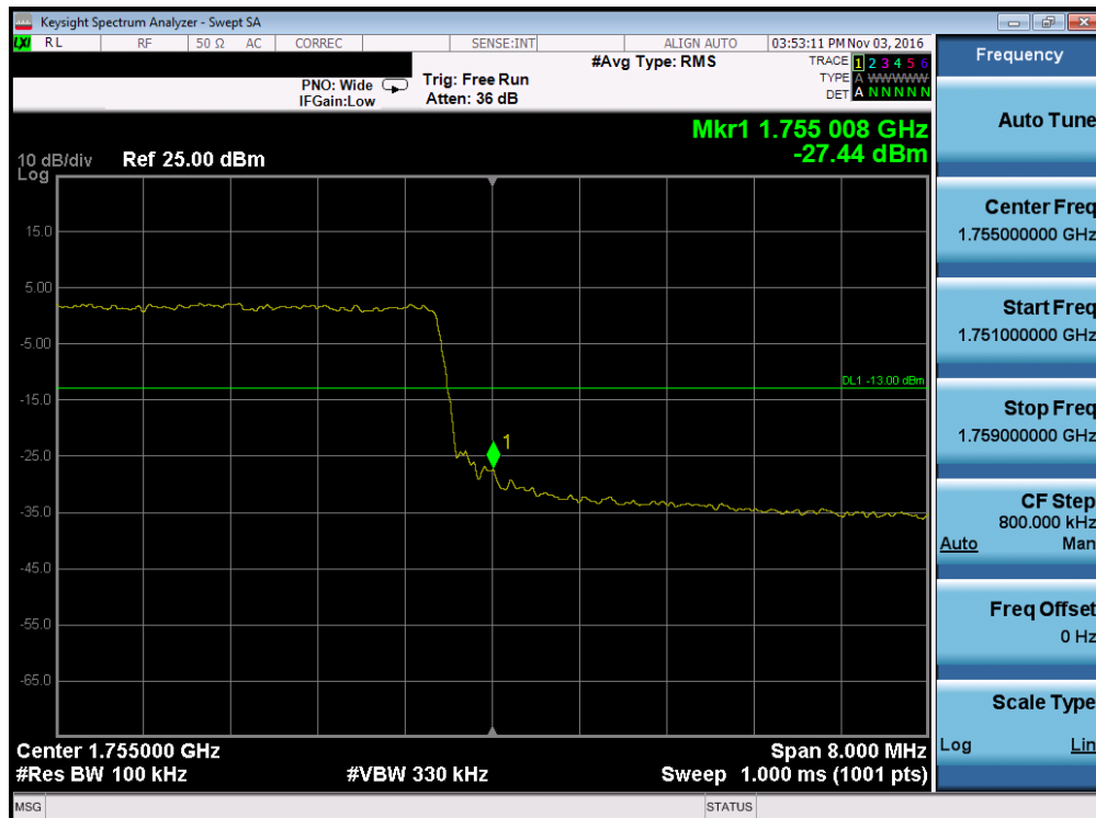
Plot 7-124. Upper Band Edge Plot (Band 4 – 10.0MHz QPSK – RB Size 50)
