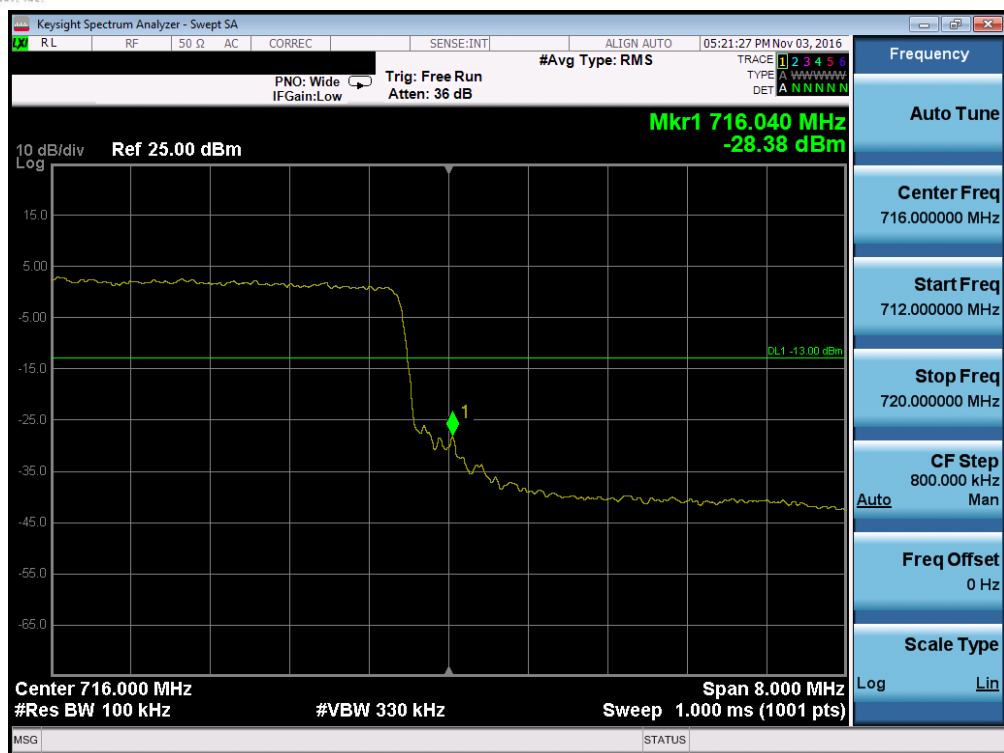
Plot 7-95. Upper Band Edge Plot (Band 17 – 10.0MHz QPSK – RB Size 50)
