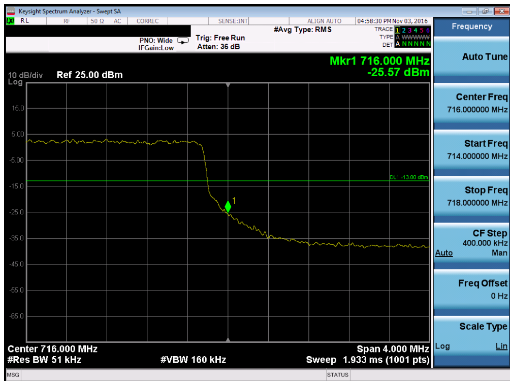
Plot 7-92. Upper Band Edge Plot (Band 17 - 5.0MHz QPSK - RB Size 25)
