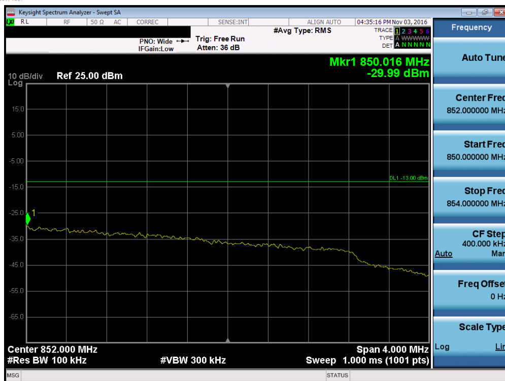
Plot 7-107. Upper Extended Band Edge Plot (Band 5 – 5.0MHz QPSK – RB Size 25)
