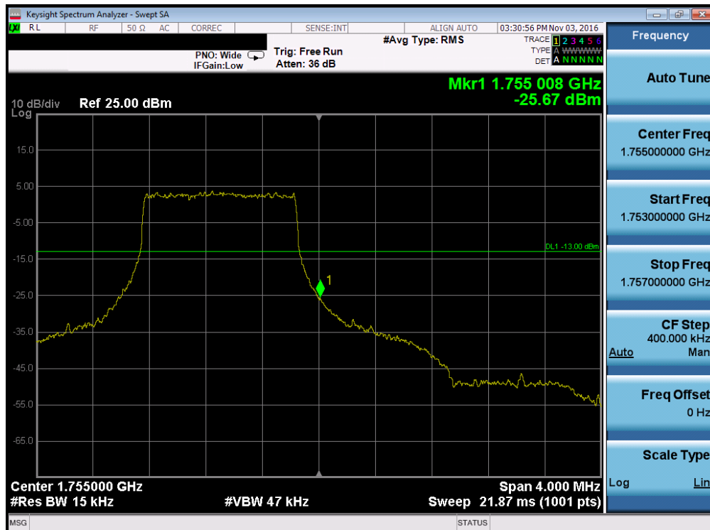
Plot 7-112. Upper Band Edge Plot (Band 4 – 1.4MHz QPSK – RB Size 6)
