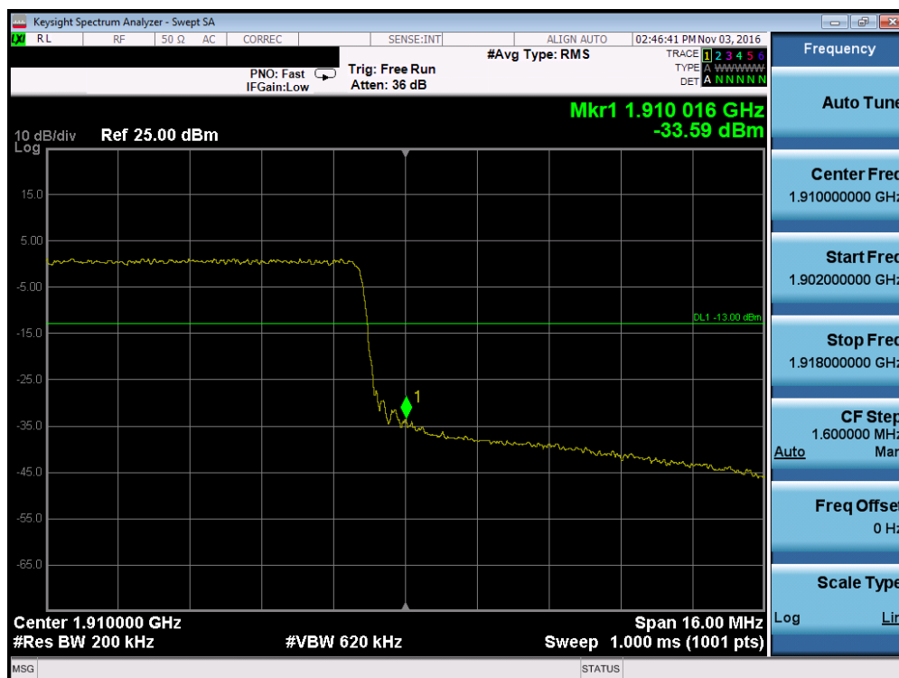
Plot 7-156. Upper Band Edge Plot (Band 2 – 20.0MHz QPSK – RB Size 100)
