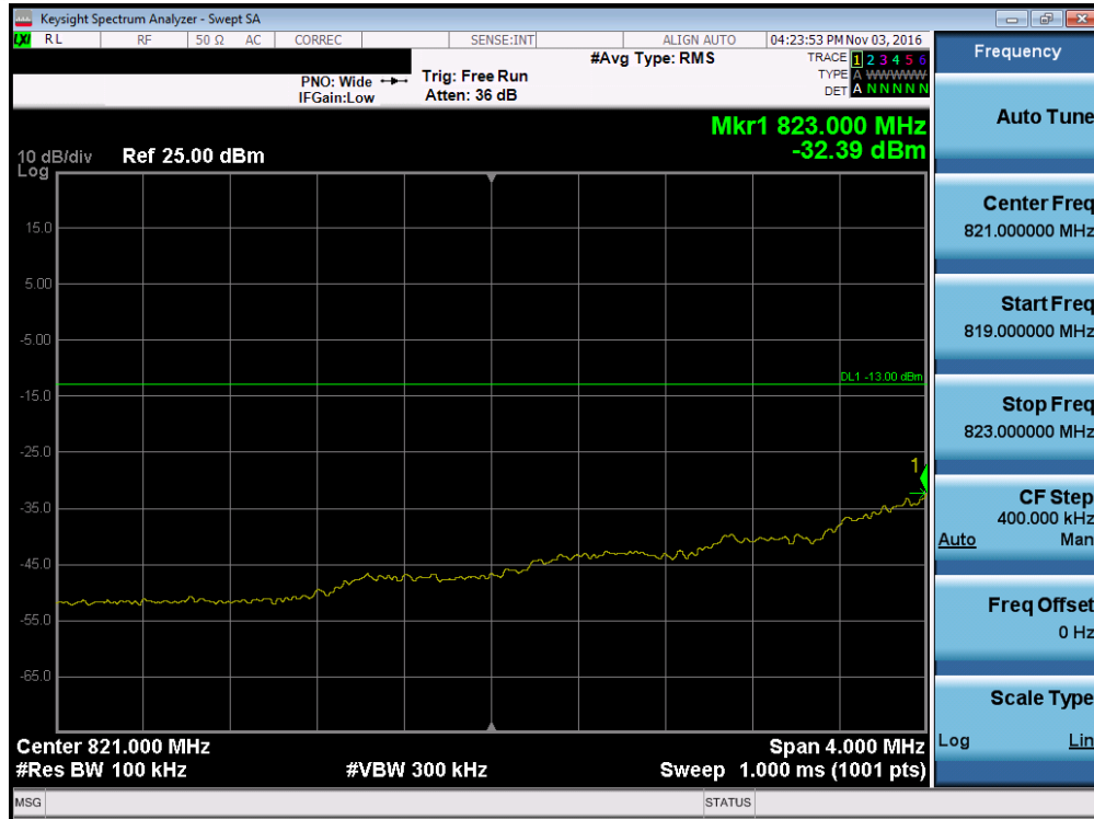
Plot 7-97. Lower Extended Band Edge Plot (Band 5 – 1.4MHz QPSK – RB Size 6)
