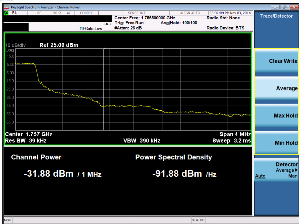
Plot 7-113. Upper Extended Band Edge Plot (Band 4 – 1.4MHz QPSK – RB Size 6)
