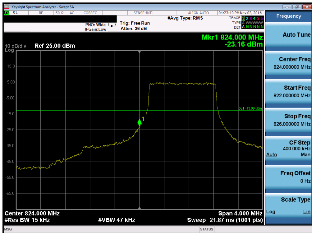
Plot 7-96. Lower Band Edge Plot (Band 5 – 1.4MHz QPSK – RB Size 6)
