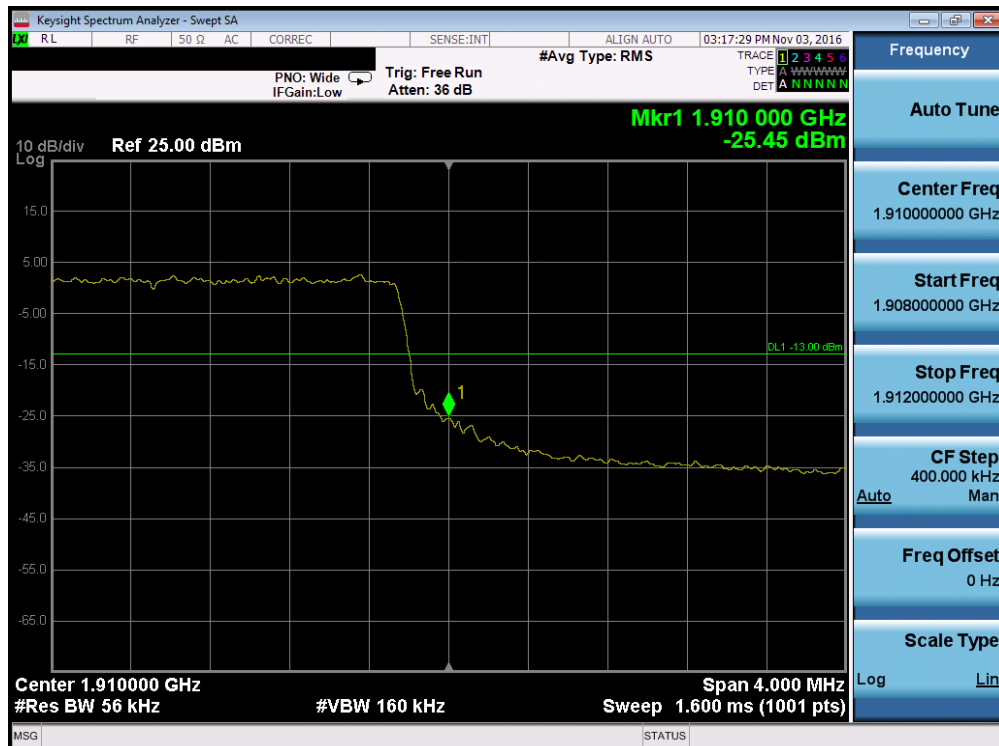
Plot 7-144. Upper Band Edge Plot (Band 2 – 5.0MHz QPSK – RB Size 25)
