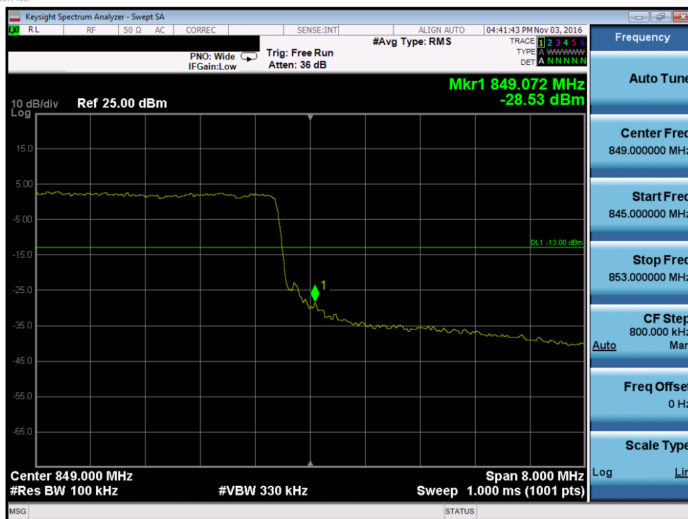
Plot 7-109. Upper Band Edge Plot (Band 5 – 10.0MHz QPSK – RB Size 50)
