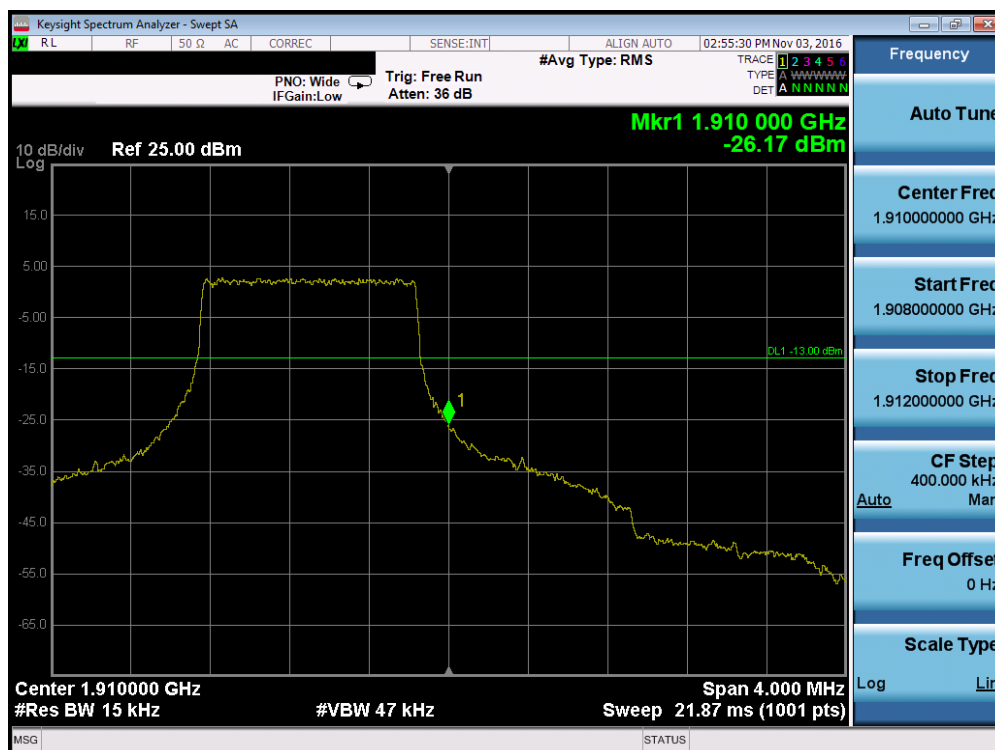
Plot 7-136. Upper Band Edge Plot (Band 2 – 1.4MHz QPSK – RB Size 6)
