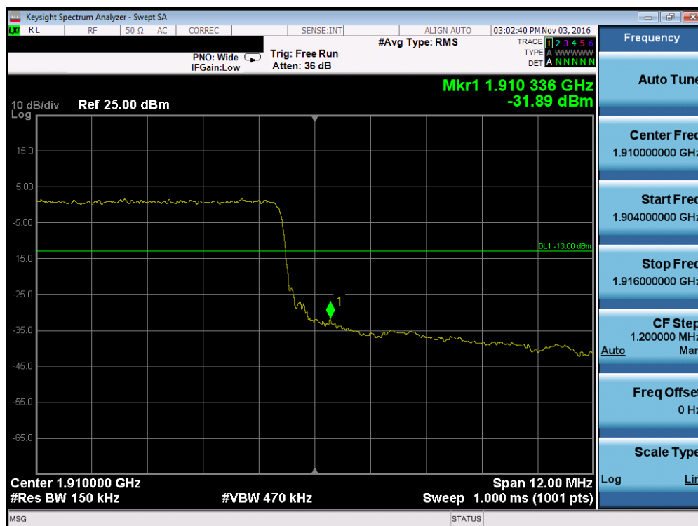
Plot 7-152. Upper Band Edge Plot (Band 2 – 15.0MHz QPSK – RB Size 75)
