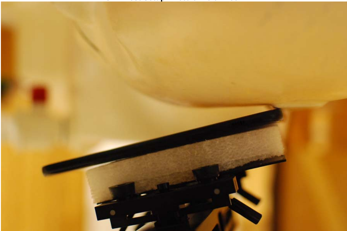
SAR Test Setup Photo 4: Left Tilt
