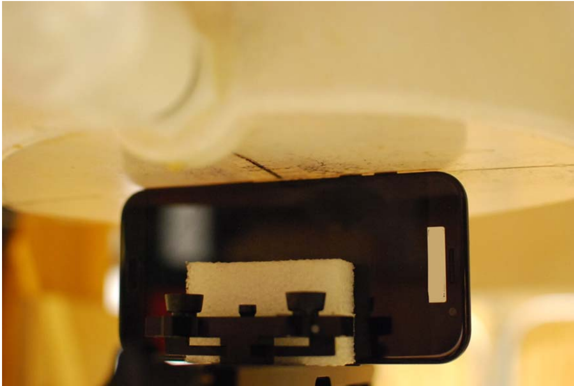
SAR Test Setup Photo 9: Left Edge at 0 mm
