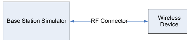
Figure 9-2 Power Measurement Setup
