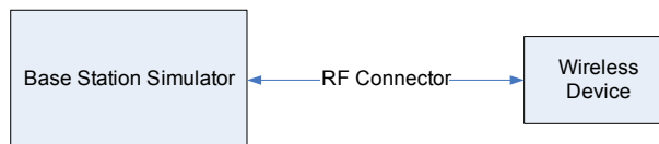
Figure 9-1 Power Measurement Setup
