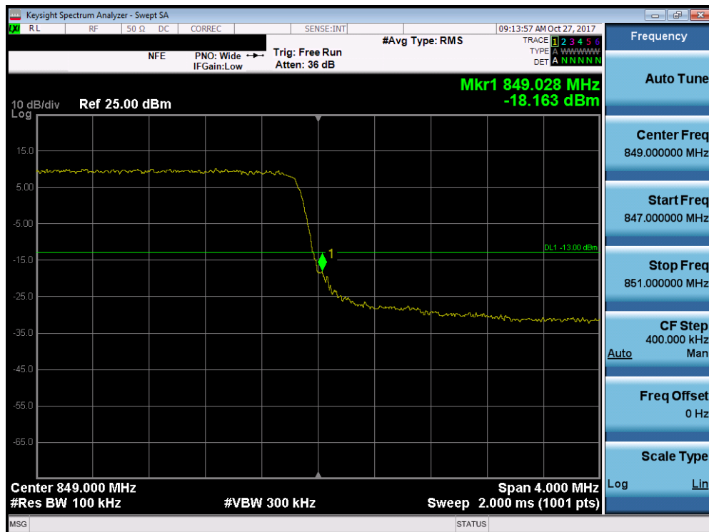
Plot 7-153. Upper Band Edge Plot (Band 5/26 - 3.0MHz QPSK - Full RB Configuration)
