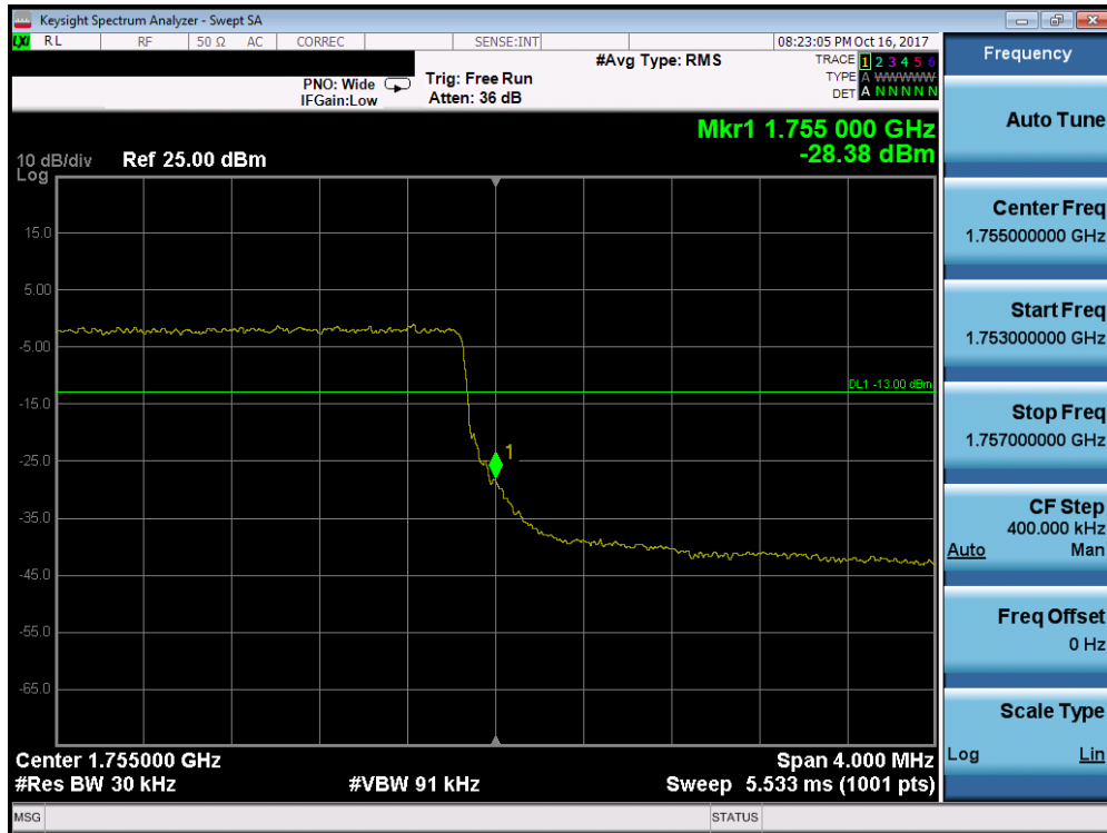
Plot 7-168. Upper Band Edge Plot (Band 4 - 3.0MHz QPSK - Full RB Configuration)
