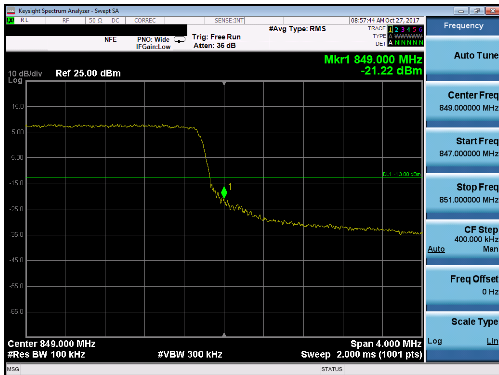
Plot 7-155. Upper Band Edge Plot (Band 5/26 - 5.0MHz QPSK - Full RB Configuration)
