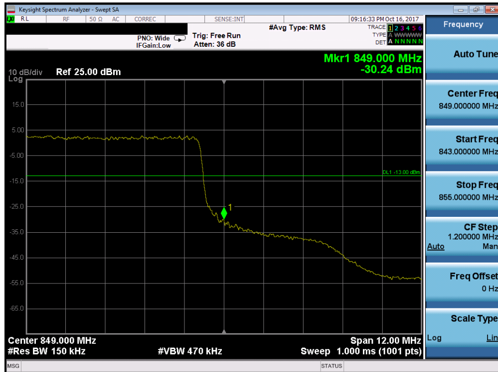
Plot 7-159. Upper Band Edge Plot (Band 26 - 15.0MHz QPSK - Full RB Configuration)
