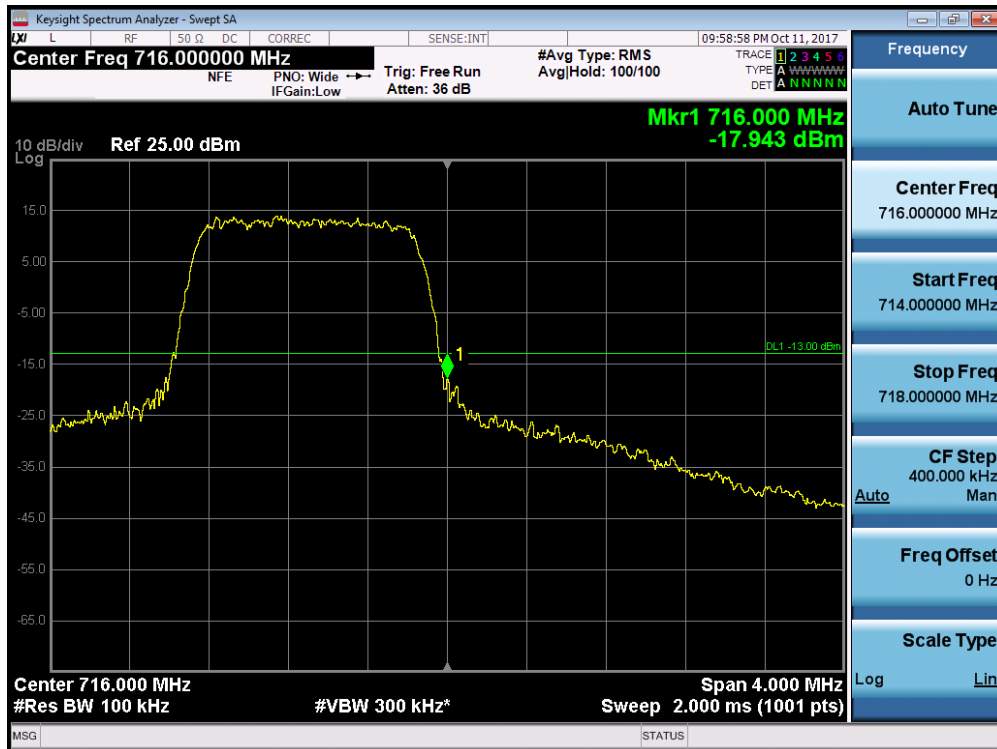
Plot 7-133. Upper Band Edge Plot (Band 12 - 1.4MHz QPSK - Full RB Configuration)
