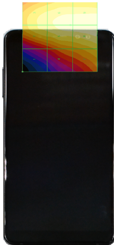
Figure 17-4 E-Field WD Scan overlay
