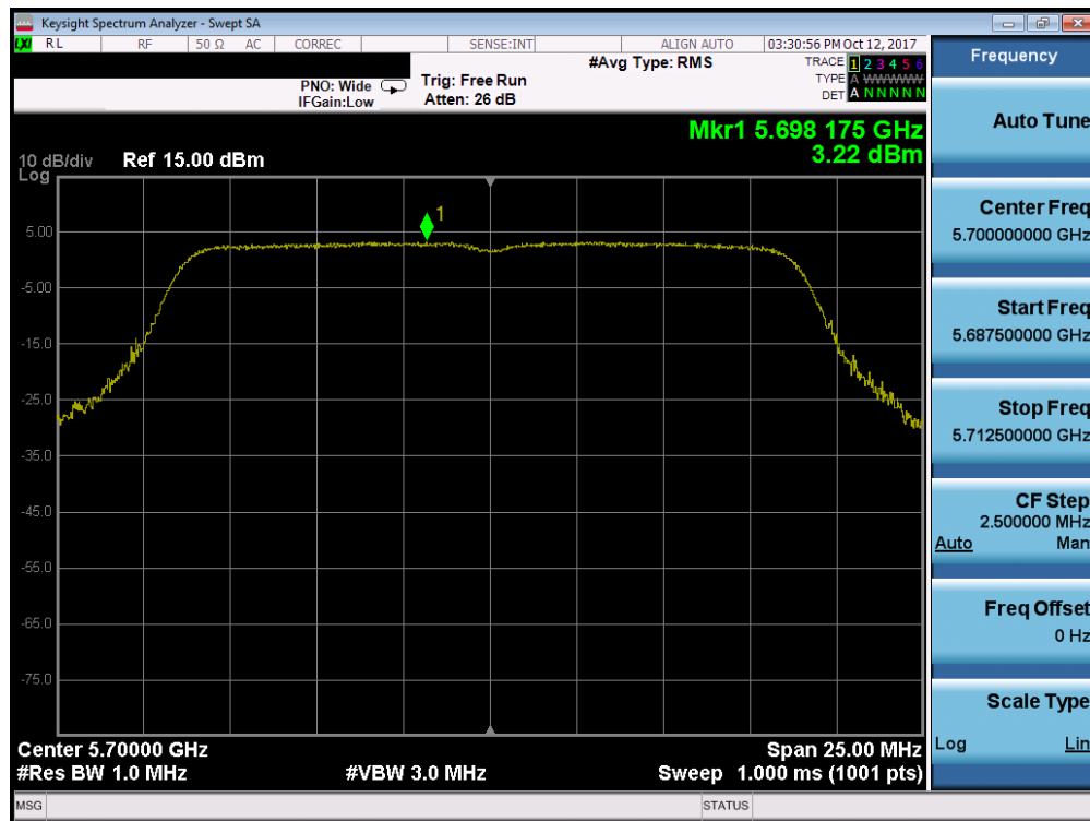
Plot 7-63. Power Spectral Density Plot (20MHz BW 802.11n (UNII Band 2C) – Ch. 144)
