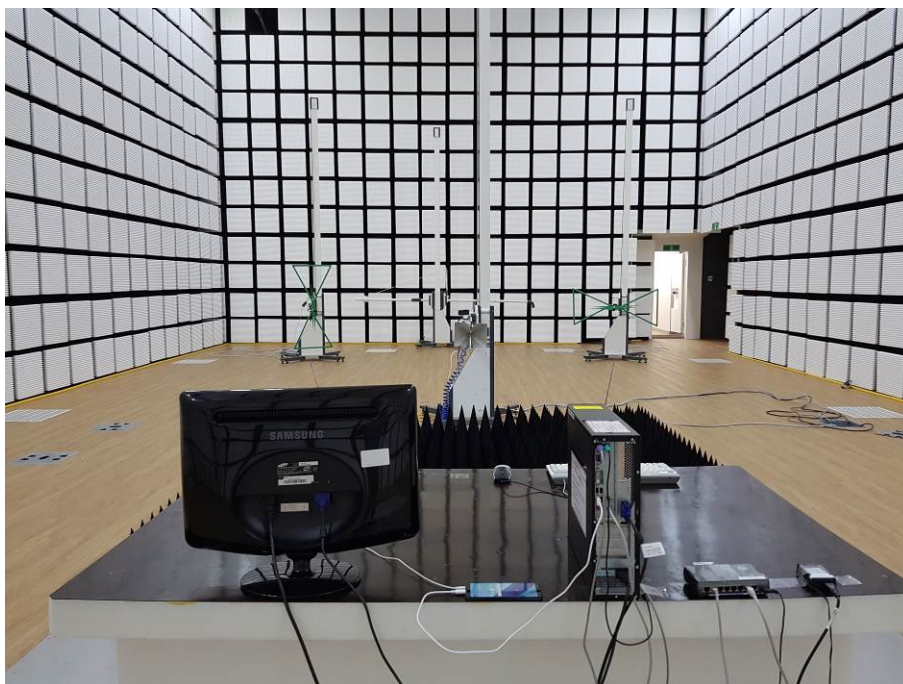
[ Radiated Disturbance for Above 1 GHz – Rear ]
