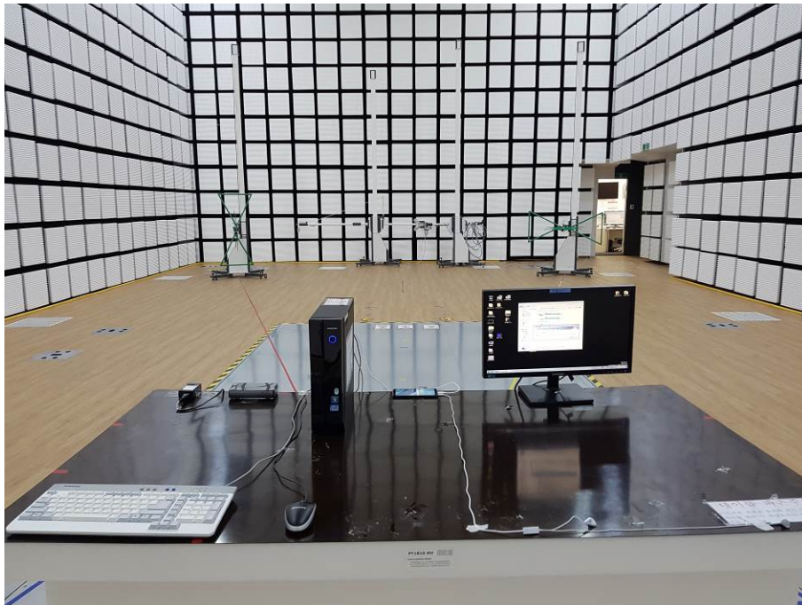
[ Radiated Disturbance for Below 1 GHz – Front ]
