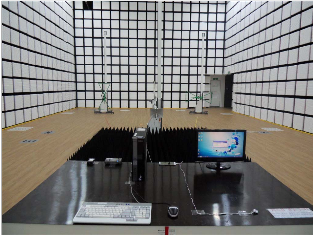
[ Radiated Disturbance for Above 1 GHz – Front ]
