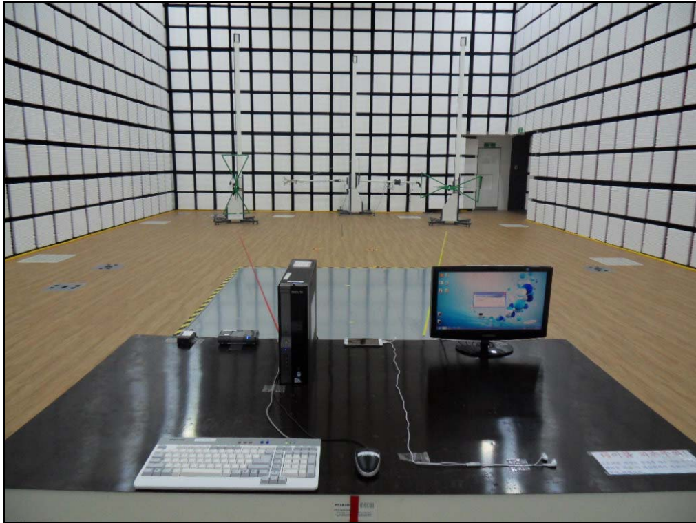
[ Radiated Disturbance for Below 1 GHz – Front ]
