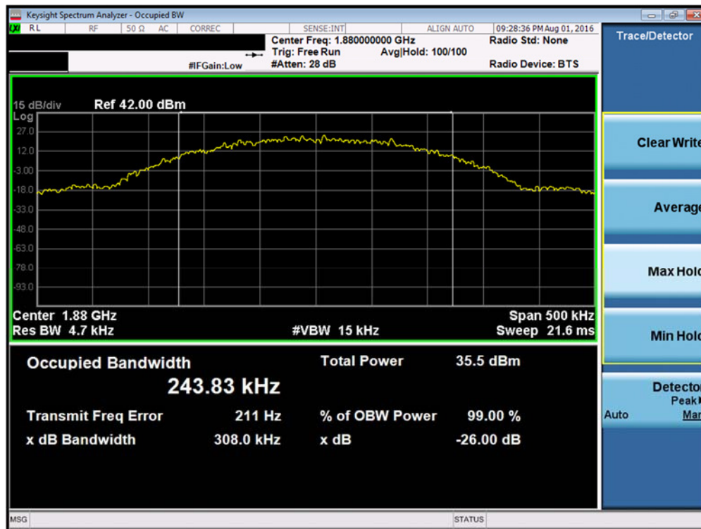
Plot 7-1. Occupied Bandwidth Plot (PCS GRPS Mode – Ch. 661)
