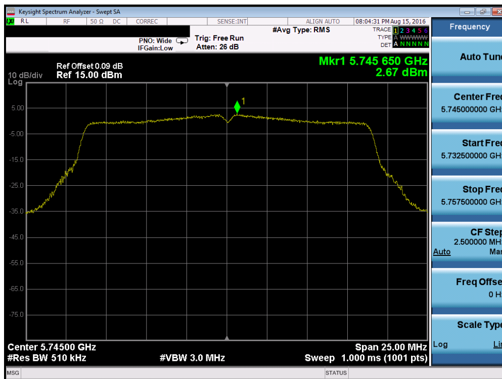
Plot 7-73. Power Spectral Density Plot (20MHz BW 802.11n (UNII Band 3) – Ch. 149)
