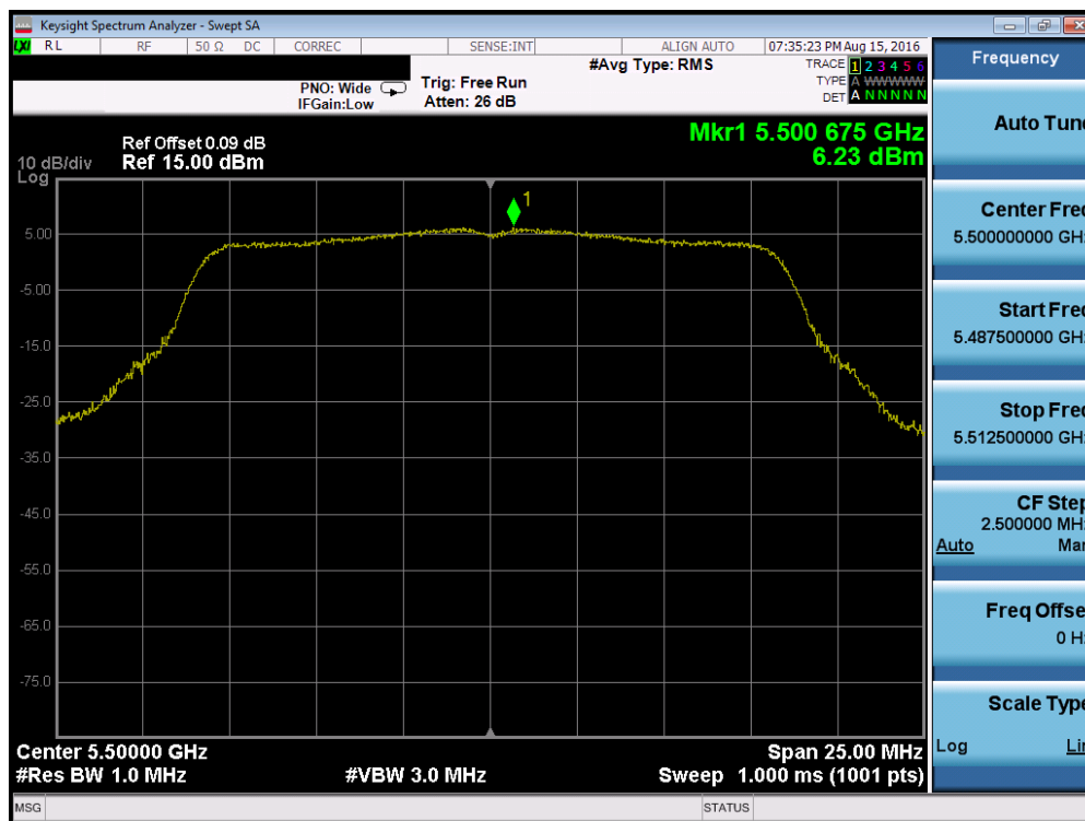
Plot 7-58. Power Spectral Density Plot (802.11a (UNII Band 2C) – Ch. 100)
