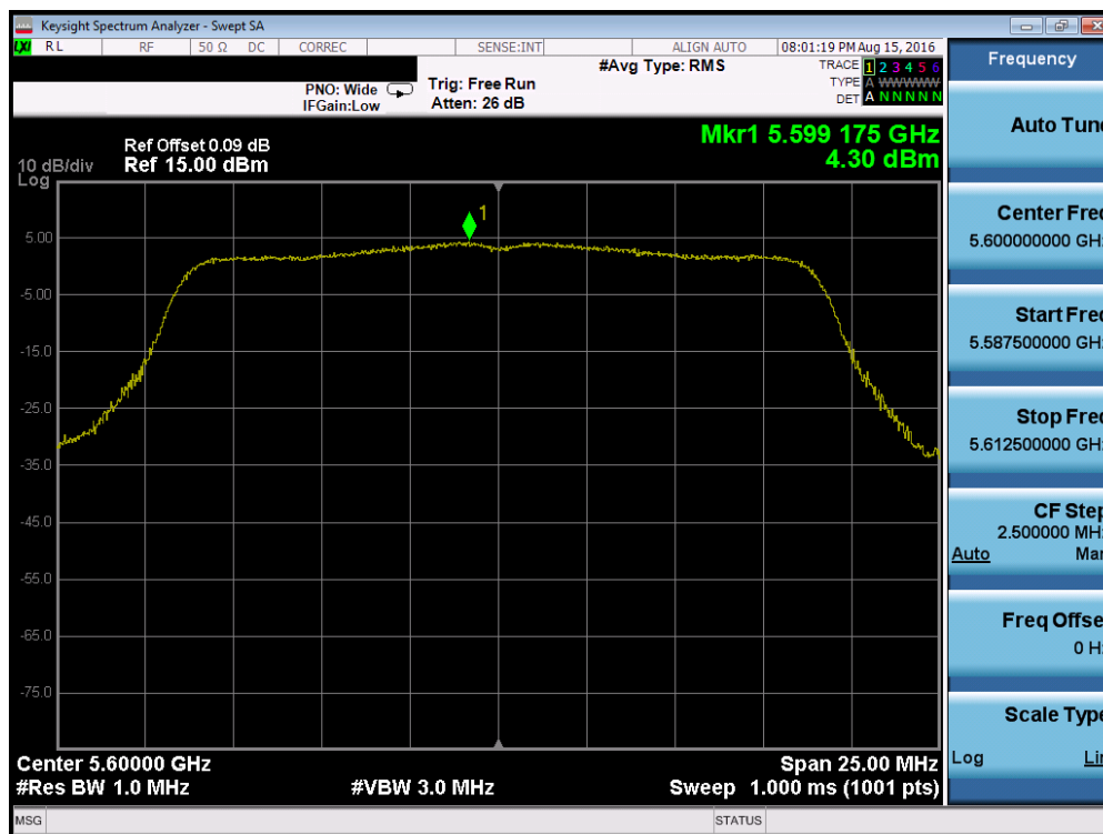
Plot 7-62. Power Spectral Density Plot (20MHz BW 802.11n (UNII Band 2C) – Ch. 120)
