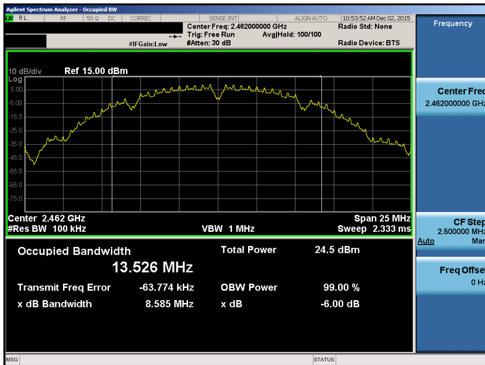
Plot 7-3. 6dB Bandwidth Plot (802.11b – Ch. 11)
