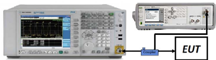
Figure 7-6. Test Instrument & Measurement Setup
