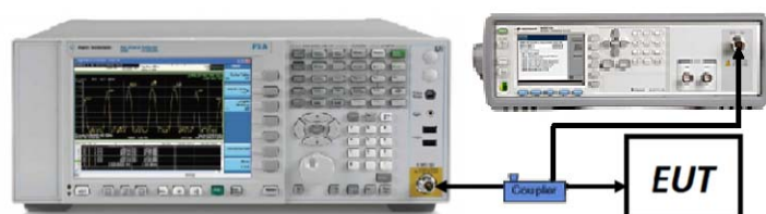
Figure 7-7. Test Instrument & Measurement Setup
