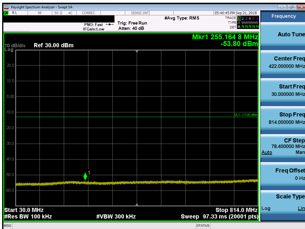
Plot 7-19. Conducted Spurious Plot (LTE Band 26, 1.4MHz QPSK – RB Size 1, RB Offset 0 – High Channel)
