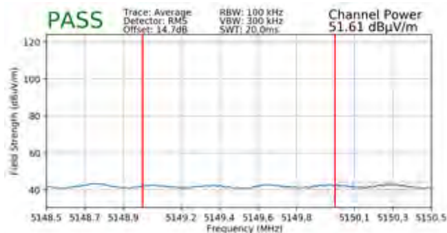
Plot 7-186. Radiated Lower Band Edge Plot SISO ANT1 (Average – UNII Band 1)
