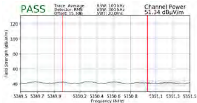
Plot 7-188. Radiated Upper Band Edge Plot SISO ANT1 (Average – UNII Band 2A)
