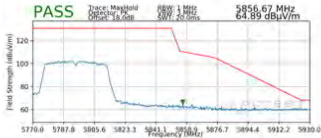
Plot 7-233. Radiated Upper Band Edge Plot MIMO (Peak – UNII Band 3)
