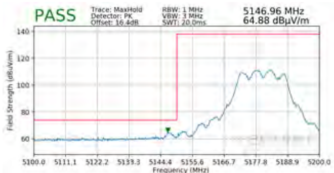
Plot 7-221. Radiated Lower Band Edge Plot MIMO (Peak – UNII Band 1)
