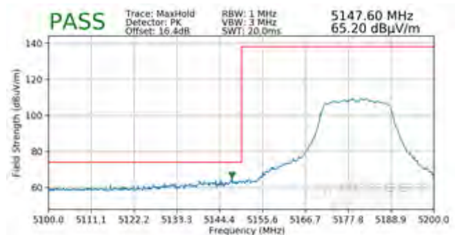
Plot 7-214. Radiated Lower Band Edge Plot MIMO (Peak – UNII Band 1)
