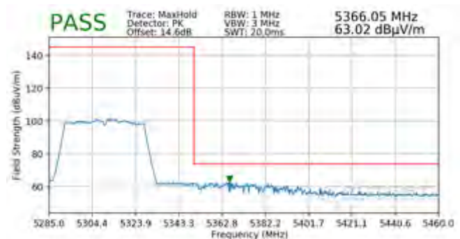
Plot 7-203. Radiated Upper Band Edge Plot SISO ANT2 (Peak – UNII Band 2A)
