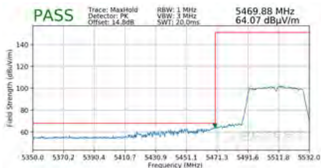
Plot 7-205. Radiated Lower Band Edge Plot SISO ANT2 (Peak – UNII Band 2C)
