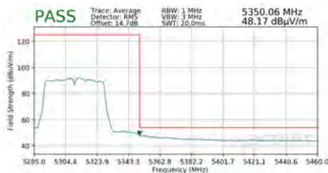
Plot 7-202. Radiated Upper Band Edge Plot SISO ANT2 (Average – UNII Band 2A)
