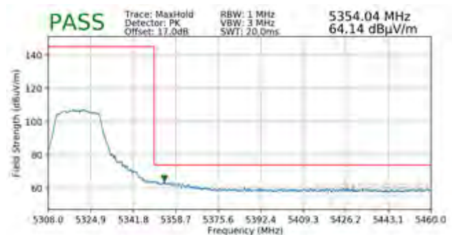
Plot 7-216. Radiated Upper Band Edge Plot MIMO (Peak – UNII Band 2A)
