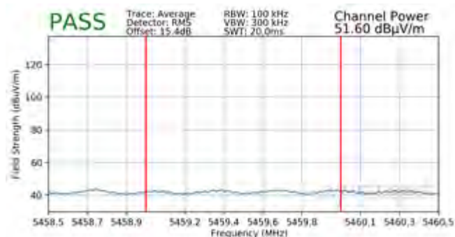
Plot 7-190. Radiated Lower Band Edge Plot SISO ANT1 (Average – UNII Band 2C)
