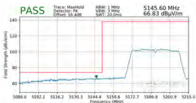
Plot 7-228. Radiated Lower Band Edge Plot MIMO (Peak – UNII Band 1)
