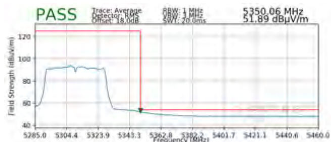
Plot 7-229. Radiated Upper Band Edge Plot MIMO (Average – UNII Band 2A)
