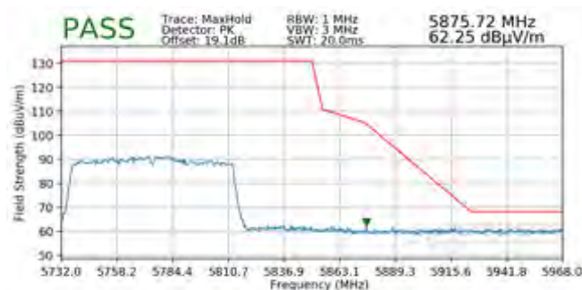
Plot 7-192. Radiated Upper Band Edge Plot SISO ANT1 (Peak – UNII Band 3)
