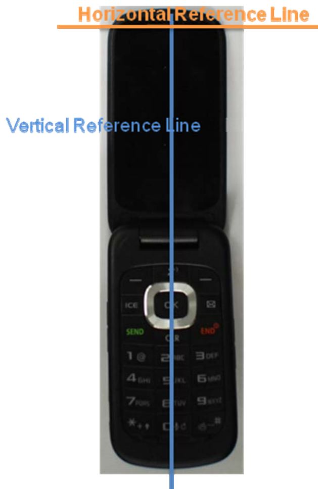
SAR Test Setup Photo 7: Horizontal and Vertical Reference Lines
