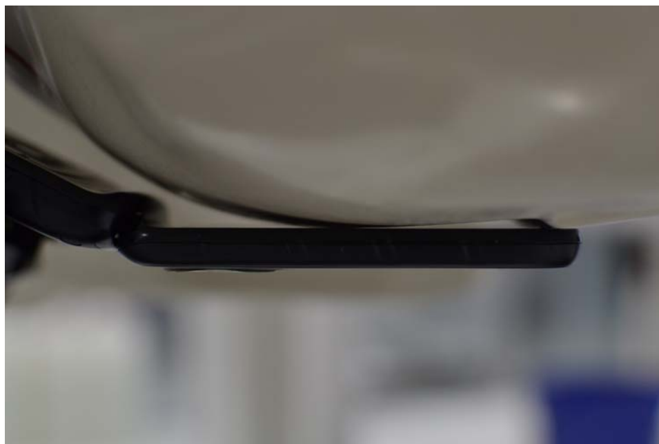
SAR Test Setup Photo 3 – Left Cheek
