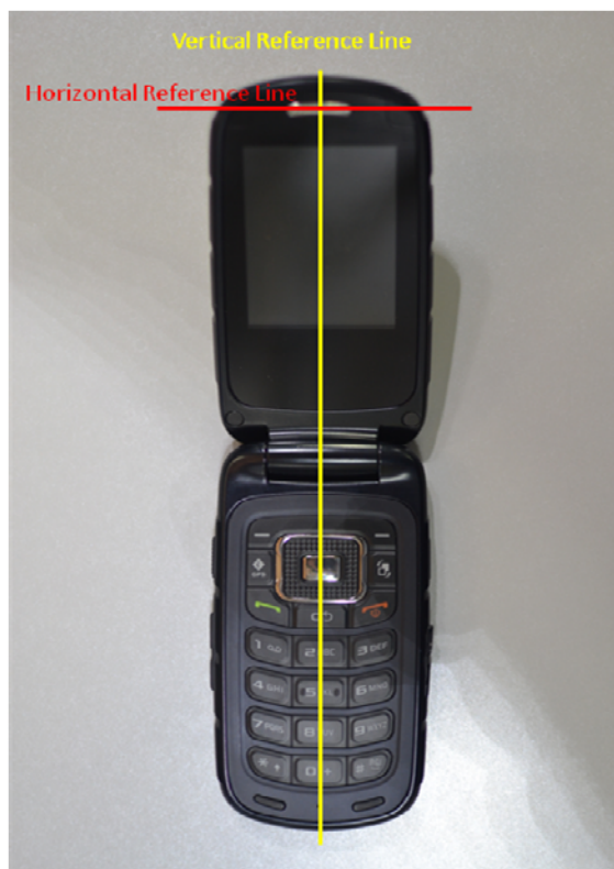
SAR Test Setup Photo 6 – Horizontal and Vertical Reference Lines
