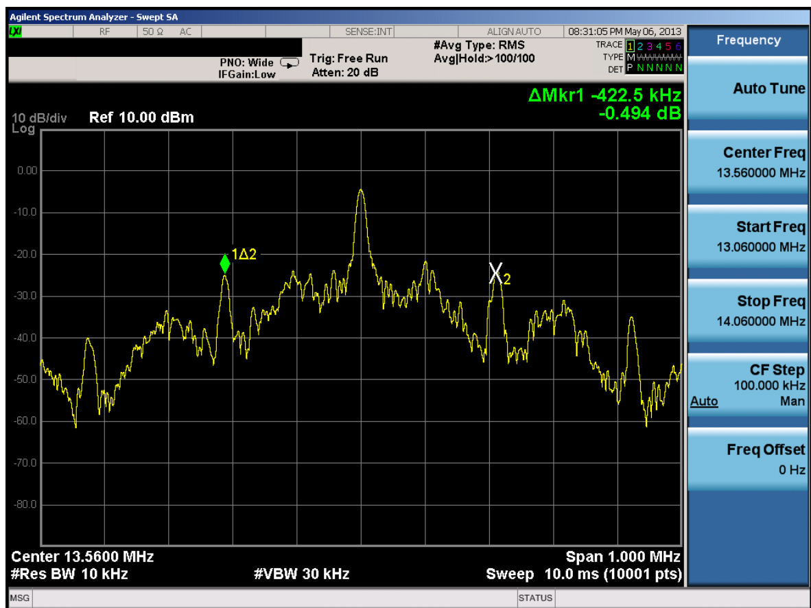
Figure 8-2. 20dB Bandwidth Plot
