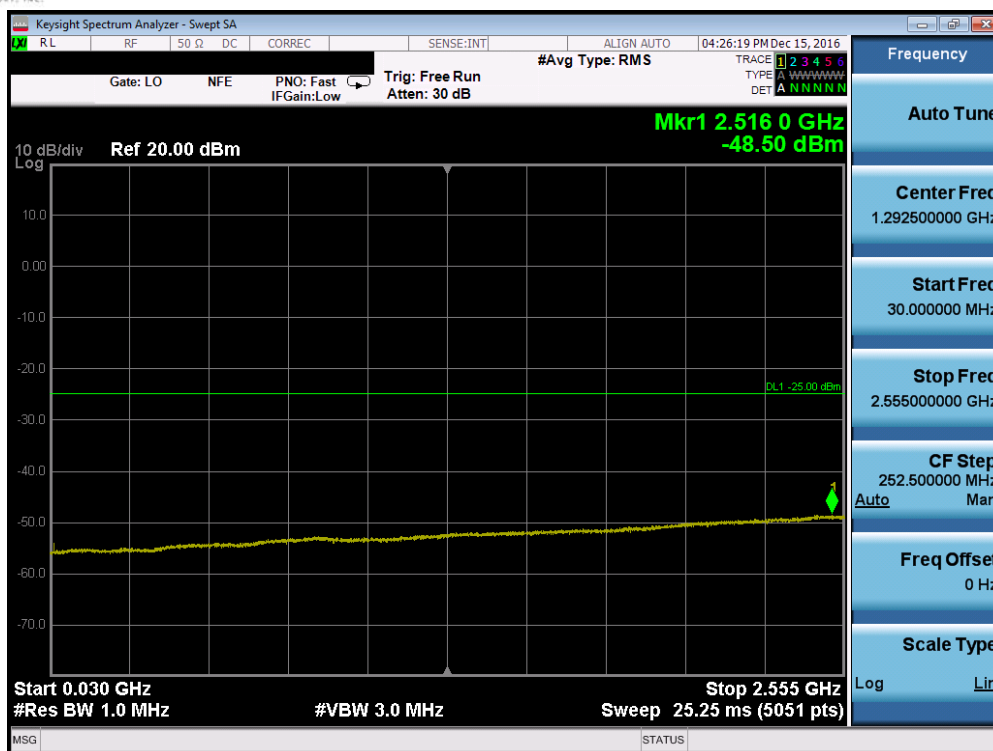
Plot 7-49. Conducted Spurious Plot (Band 41 – 5.0MHz QPSK – RB Size 1, RB Offset 0 – Mid Channel, Antenna-C)
