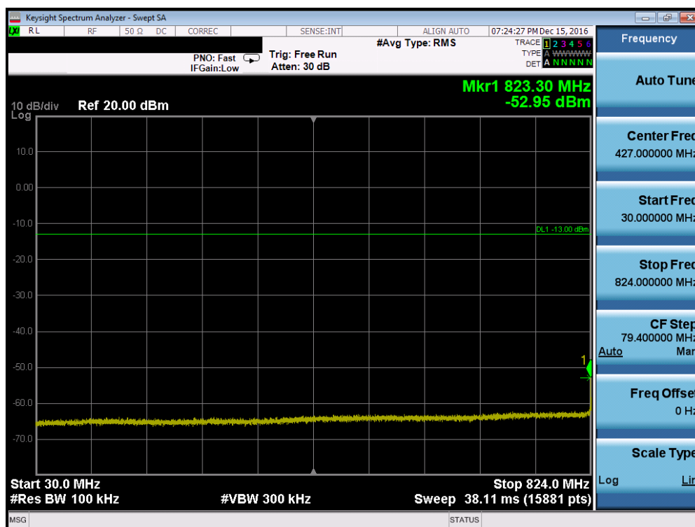
Plot 7-58. Conducted Spurious Plot (Band 5 – 10.0MHz QPSK – RB Size 1, RB Offset 0 – Mid Channel, Antenna-B)
