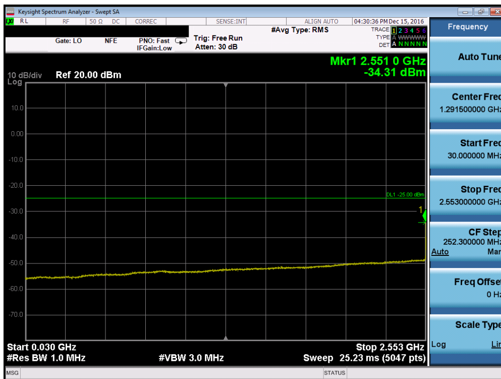
Plot 7-46. Conducted Spurious Plot (Band 41 – 5.0MHz QPSK – RB Size 1, RB Offset 0 – Low Channel, Antenna-C)
